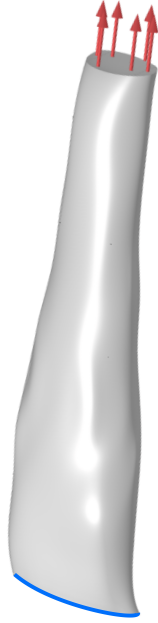
Fig. 7: On the most proximal face of the Achilles tendon FE model, the estimation of the force produced by the triceps surae muscle was applied, evenly distributed over the surface. The most distal face of the model (blue) was fixed on its place.
