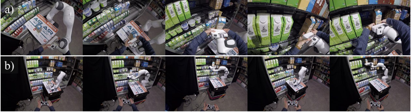
Fig. 2. The learning flow in teaching a robot how to perform item reshelfing.; beginning with a single demonstration in a), followed by multiple rounds of correction in after which the robot is able to autonomously carry out the task as depicted in b).
