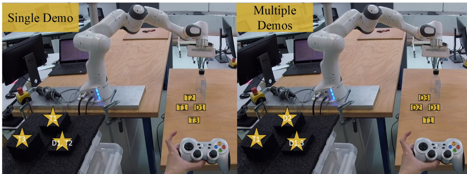
Figure 4.3: The experimental setup. Object and corresponding goal locations used for the demonstrations are denoted by D, whereas the object and goal locations used for the evaluation are denoted by T. While object locations are only varied in the plane, goal locations are varied within the 3D space.
