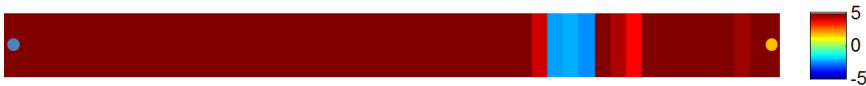
Figure 4.4: Updated permeability field of the 1D reservoir model for experiment #2. Permeability values are expressed as the natural logarithm of permeability in mD.
