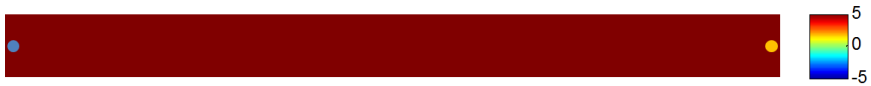
Figure 4.2: Permeability field of the starting model. Permeability values are expressed as the natural logarithm of permeability in mD. The blue and orange dots indicate the injector and the producer respectively.
