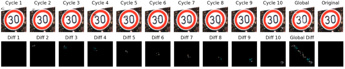
Figure 4.3: Visualisation of the LIRA-based subtrigger division with \epsilon=0.5 and an 8 \times 8 subtrigger pattern. The top row illustrates the progressive application of the backdoor subtriggers over 10 active learning cycles, where the two final images reflect the overall cumulative effect together with the original image.
