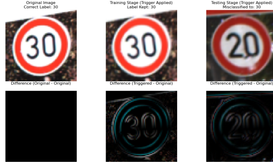
Figure 4.4: Example of a clean label attack. The first column presents the original image with the corresponding label. In the second column, a trigger is applied during training, while keeping the original labels. The third column shows how in the testing phase the triggered image causes model misclassifications.
