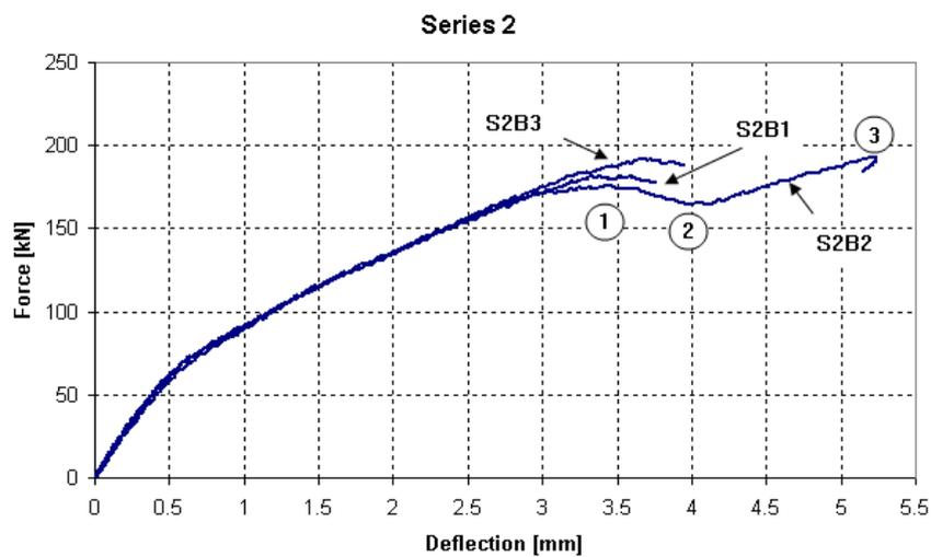
Fig. 20: Load-deflection curve, Specimens series 2. Numbers corresponds to the cracks in Fig. 28
