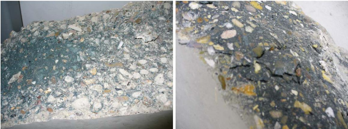
Fig. 18: Surface of crack in NSC (Left) and HSC beam (Right)
