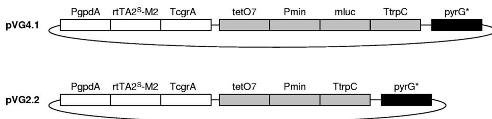
FIG. 1. The Tet-on system for A. niger . Plasmid pVG4.1 comprises one module ensuring constitutive expression of the tetracycline-dependent transactivator (PgpdA::rtTA2 S -M2::TcgrA, with the A. nidulans PgpdA promoter and the A. fumigatus crgA terminator), a second module enabling mluc reporter gene expression in an rtTA2-M2-dependent manner (tetO7::Pmin::mluc::TtrpC, with tetO7::Pmin as an rtTA2 S -M2-dependent promoter and the A. nidulans trpC terminator), and a third module, pyrG * , necessary for homologous integration of the plasmid at the pyrG locus of A. niger . The control plasmid pVG2.2 is identical to pVG4.1 but lacks the mluc gene. For cloning details and plasmid and fragment sizes, as well as restriction endonuclease sites, see Fig. S1 in the supplemental material.
