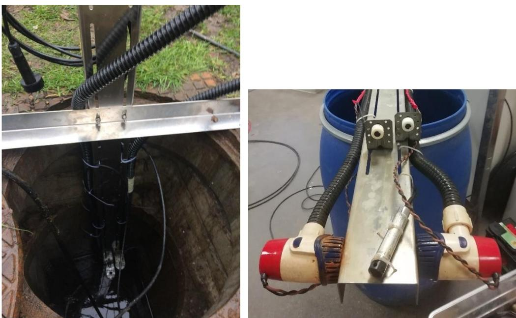
Figure 53: Frame in manhole; Pumps, level stick and floaters of the discharge measuring device
