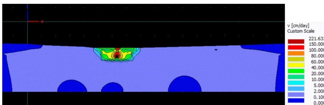
Figure 26: Bioswale E, flow velocities 0.36 days into the storm simulation
