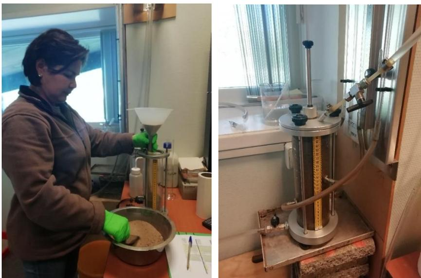
Figure 25: Pictures  $K_s$ -test disturbed samples in laboratory
