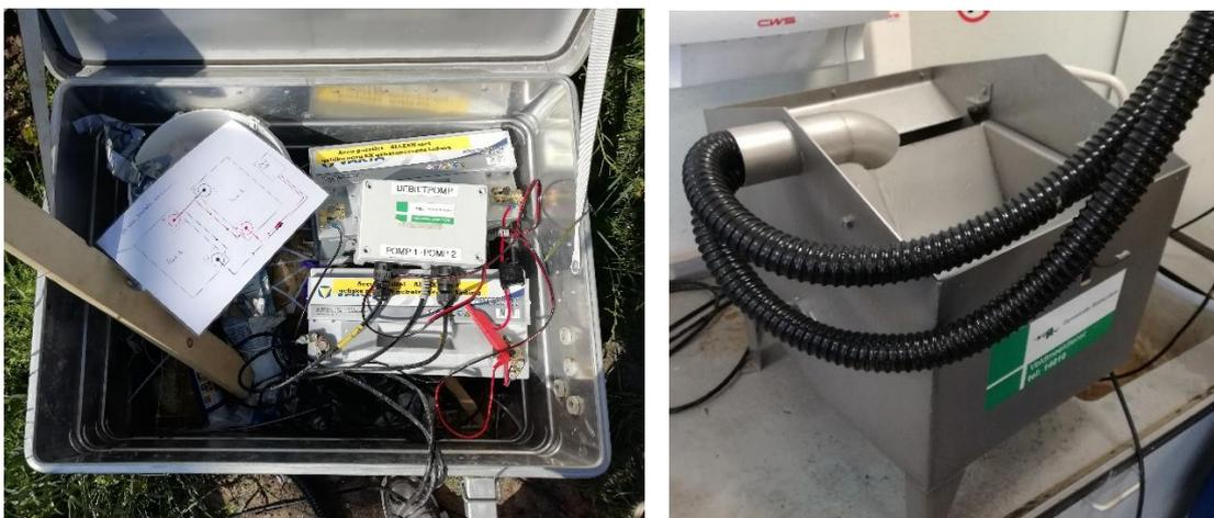
Figure 54: Chest with control box and batteries inside; Tipping counter in laboratory set-up
