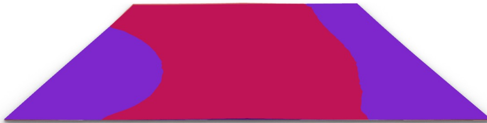
(a) Imperfect plate geometry of 3D scan (red) and DIC (purple) for experiment 2 (WAAM)
