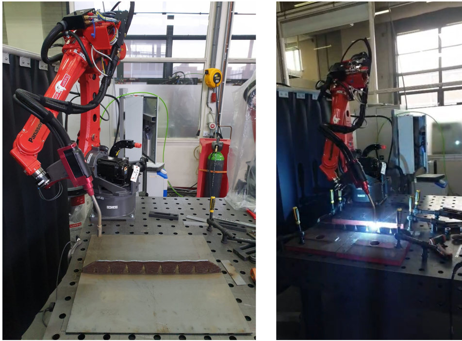
Figure 3.2: The WAAM machine used for the manufacturing of the stiffeners
