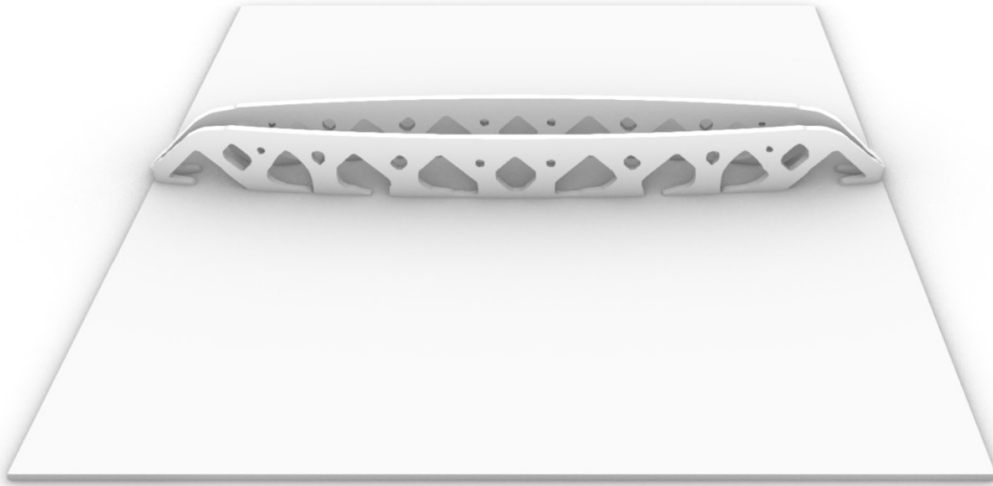
Figure 4.31: 3D model of the final stiffener geometry, including plate and stiffener thickness
