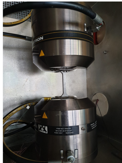
Figure 3.10: The coupon dimensions (left) and the tensile testing setup (right)
