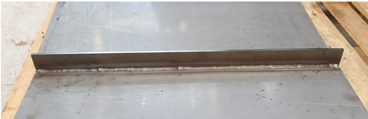
Figure 3.6: Finalized prismatic rectangular stiffener specimen
