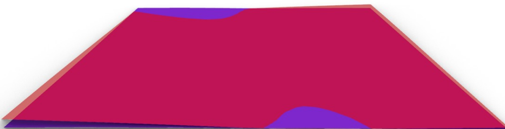
(b) Imperfect plate geometry of 3D scan (red) and DIC (purple) for experiment 3 (prismatic)
