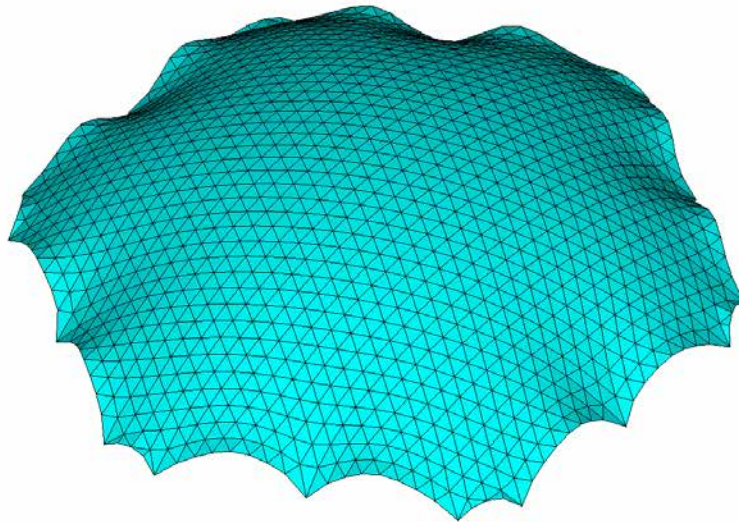
(b) Initial conditions of Example 5.2 with more point supports and the Form-Finding result.
