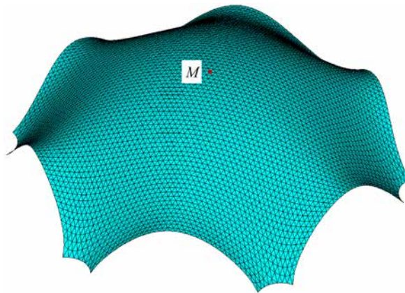
FIGURE 8.18 Model D (shell with strongly inward-curved supports).
