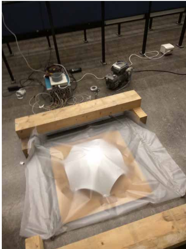
FIGURE 9.8 Manufacture of the vacuum bag.
