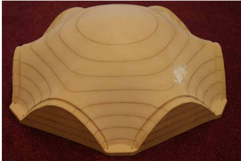
(c) Formwork of Model C (shell with inward supports).
