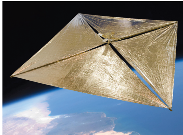
Figure 2.7: Square solar sail of the NanoSail-D spacecraft. [18]
