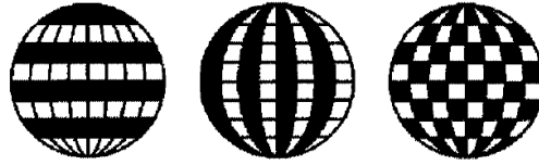
Figure 3.6: Spherical harmonics describing the deviation from a perfect sphere, from left to right: zonal, sectorial and tesseral harmonics. [24]
