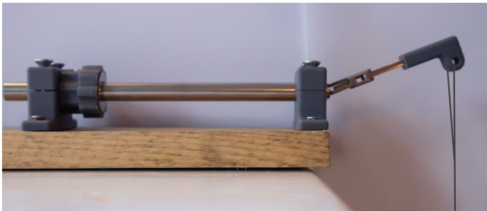
Figure 4: Test setup for the force test. The prototype is secured in a holder, and a weight of 5N is placed at the end of the fans.
