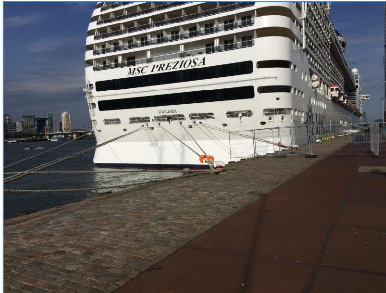
Figure 64: Mooring pattern of the MSC Preziosa at the Holland America cruise terminal (photo 20/09/2017)
