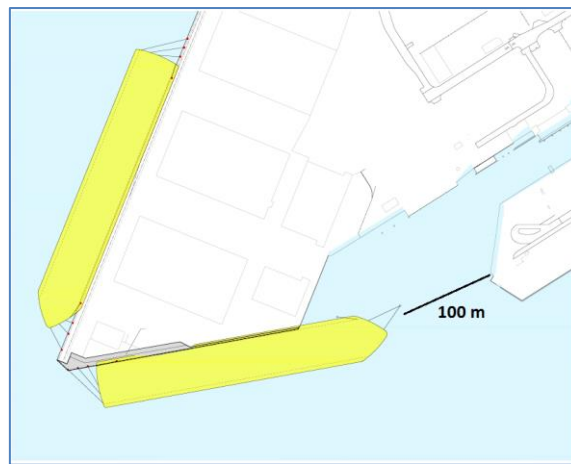
Figure 27: New quay wall with mooring dolphin at the riverside Pier 1
