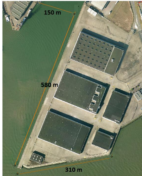
Figure 8: Main dimensions of Pier 1 in the Merwehaven (Globespotter)
