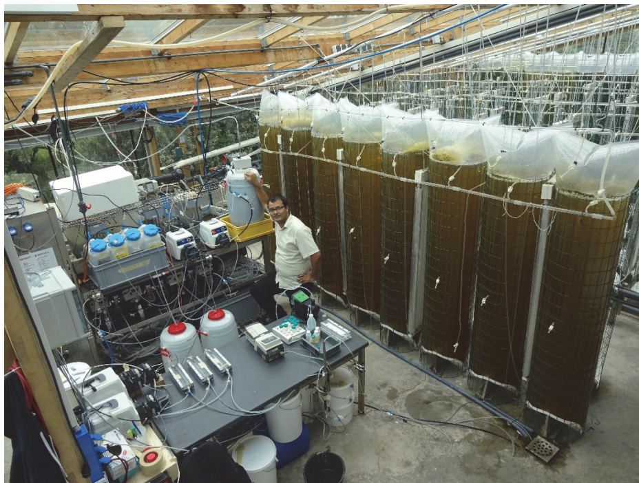
Supplementary Figure S.5.3: General overview of a pilot plant in Zeeland, Jacobahaven, the Netherlands. The large plastic bags are the algal culture of marine diatom Chaetoceros affinis
