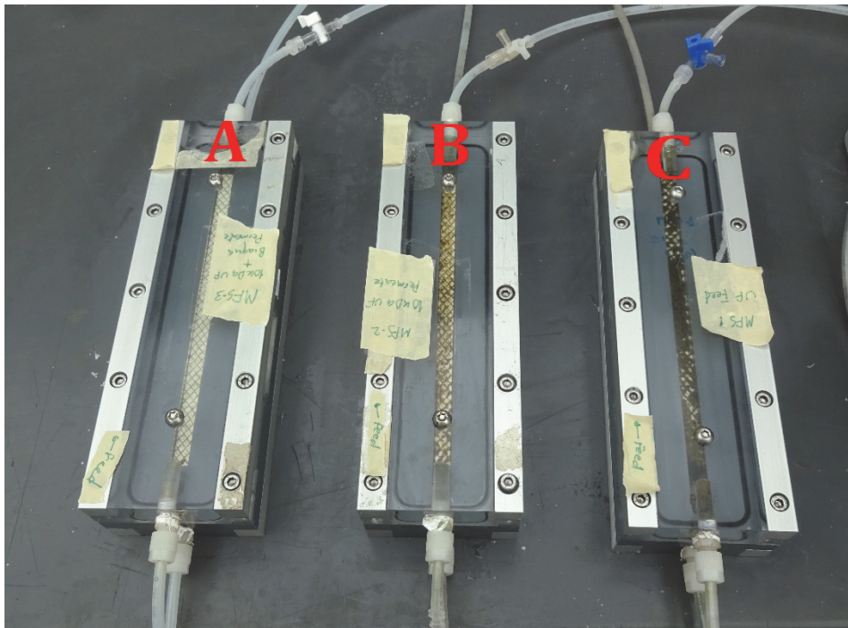
Supplementary Figure S.6.1: Three MFS cells on operation fed with A) 10 kDa UF+PRT™ permeate, B) 10 kDa UF permeate, and C) UF feed
