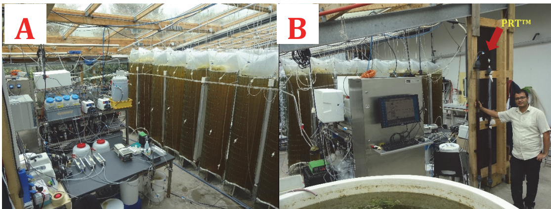
Supplementary Figure S.6.2: A) General overview of a pilot plant in Zeeland, Jacobahaven, the Netherlands. The large plastic bags are the algal culture of marine diatom Chaetoceros affinis B) PRT™ column packed with phosphate adsorbent
