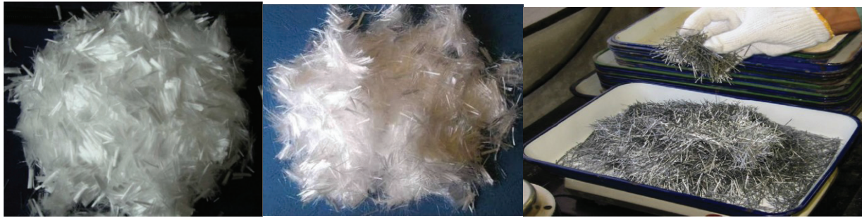
Figure 2. Photo on the left: Polyvinyl Alcohol (PVA) fibres [17]. Photo in the centre: High Modulus Polyethylene (HMPE) fibres [18]. Photo on the right: steel fibres [19]
