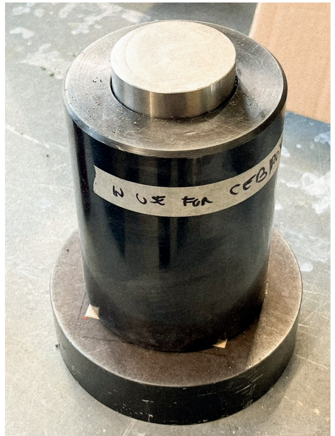
Figure 64: Stainless-steel plunger inserted 40 mm into the mixture, ensuring guided alignment within the mould before compaction.
