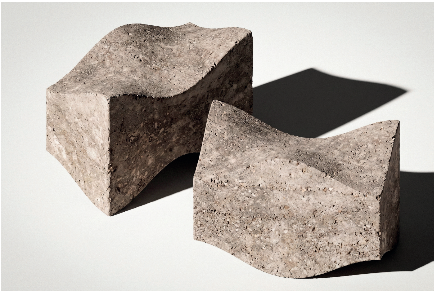
Figure 115: AI-assisted visualisation of exploratory osteomorphic-inspired compressed earth blocks based on the investigated excavation material.
