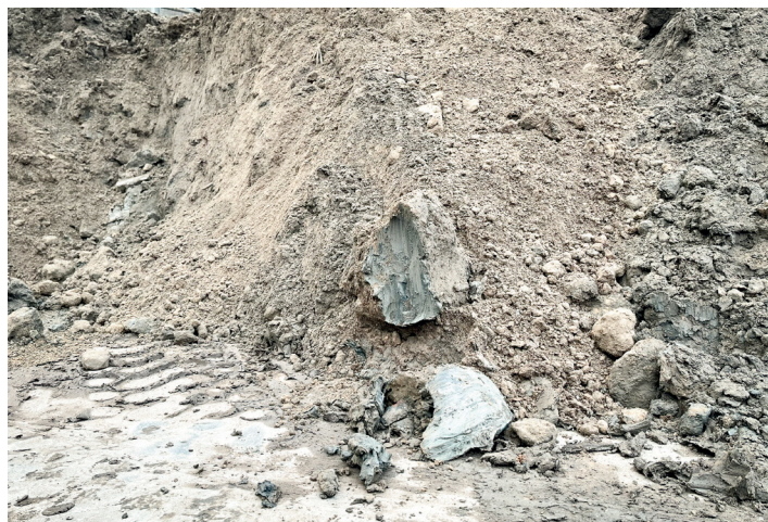
Figure 08: Deposited excavation material, characterised by large cohesive clay clods.
