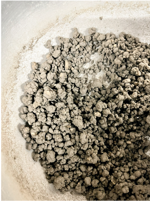
Figure 77: Mixture at the processing limit, showing severe clumping during mixing.
