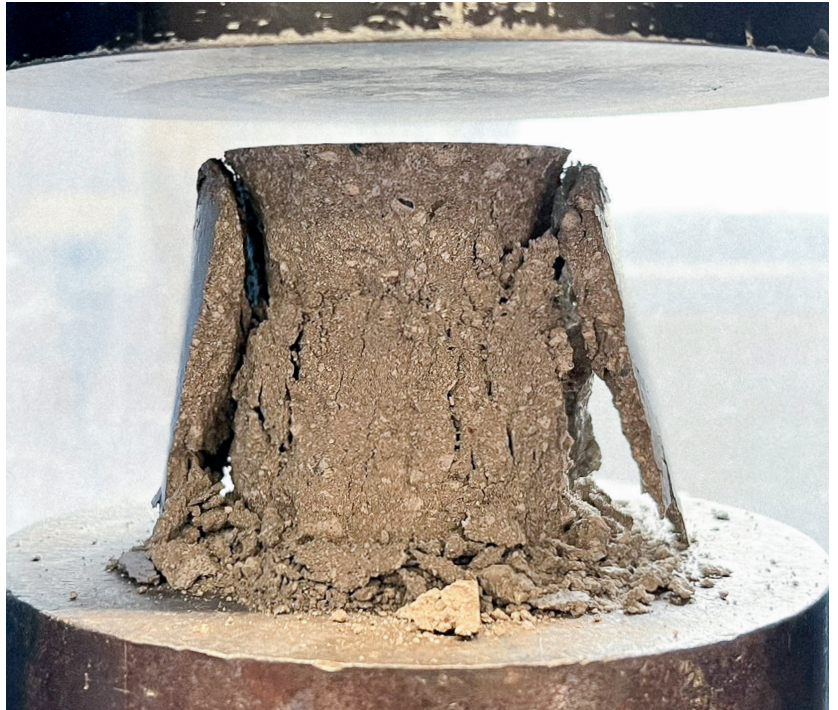
Figure 68: Shell-like detachment of outer layers from the specimen edges after failure.
