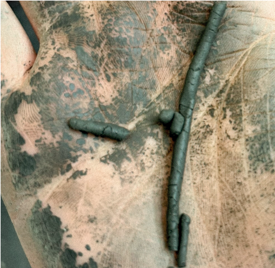
Figure 15: Manual plasticity assessment showing cracking and crumbling of the soil thread at the rolling limit.
