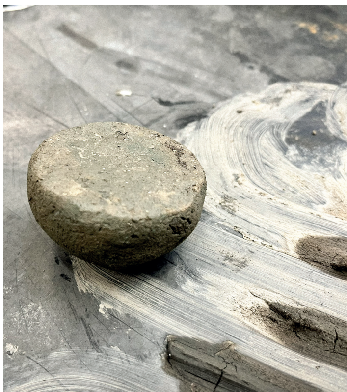
Figure 10: Spherical clay sample after drop test.
