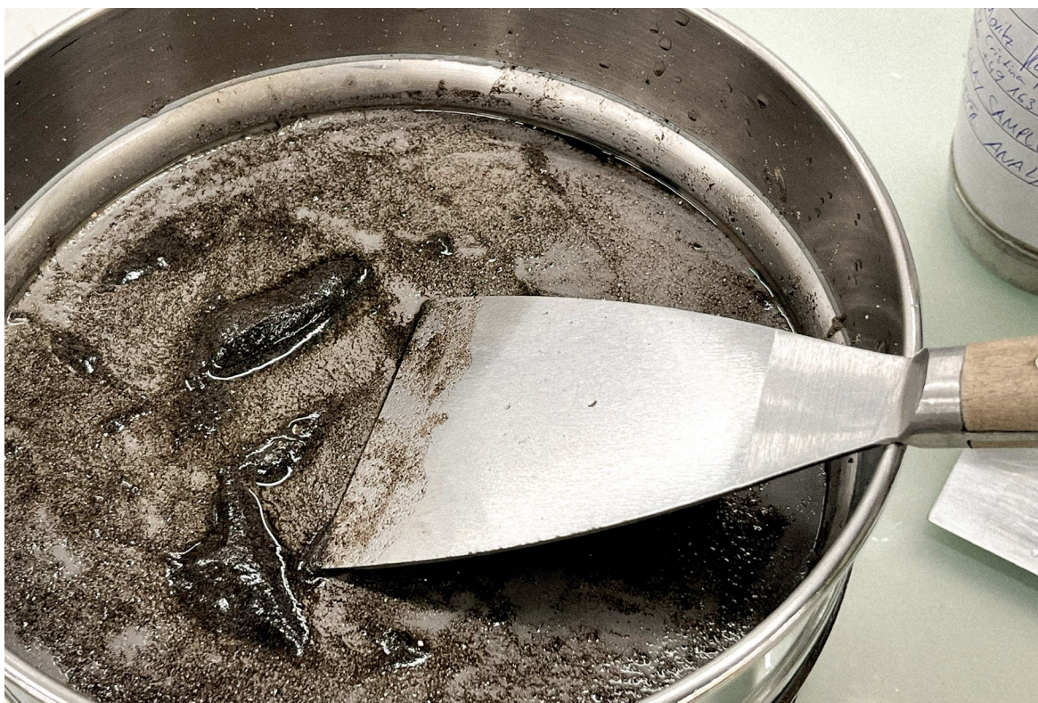
Figure 18: Wet sieving of the dispersed sample through a 0.063 mm sieve, using a spatula and distilled water to separate the sand fraction.
