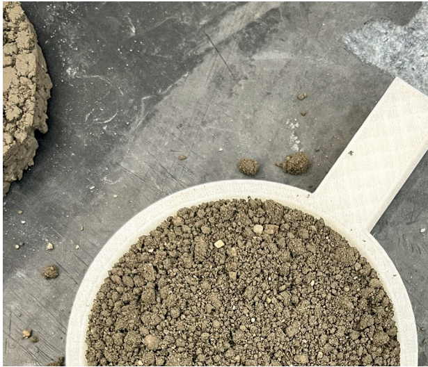
Figure 57: 3D printed preliminary mould.
