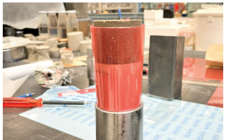
Figure 75: Successful release of the specimen using FPCR inlay.
