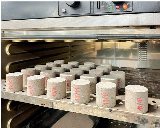
Figure 79: Specimen series oven-dried at 60 °C to avoid alteration of the mineralogical composition.
