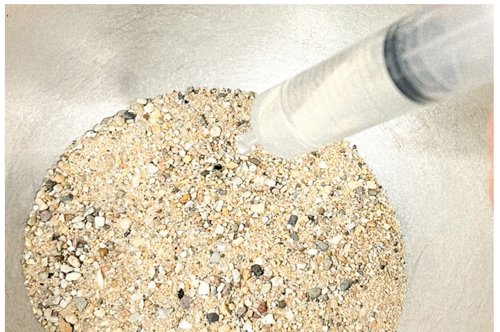
Figure 54: Stepwise water addition using a syringe.
