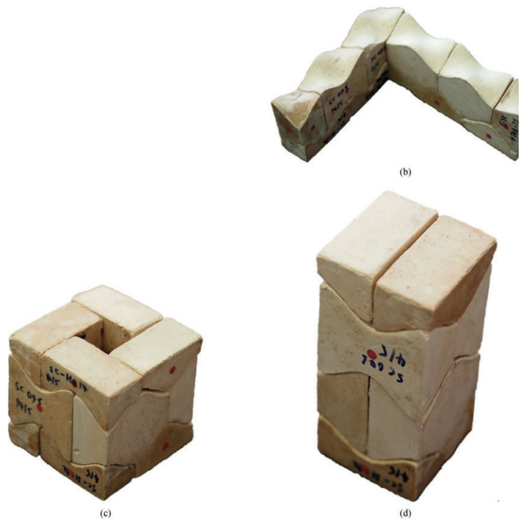
Figure 114: Examples of structures that can be assembled from osteomorphic blocks. Reproduced from Dyskin et al. (2012).
