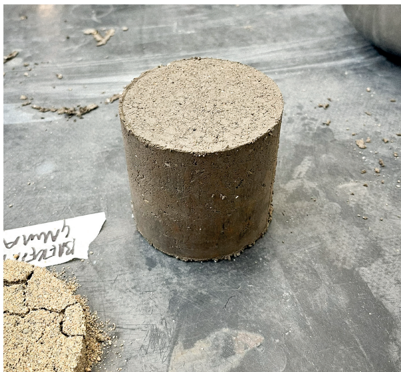
Figure 62: Freshly demoulded specimen after compaction.
