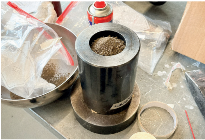
Figure 63: Filled mould prior to compaction.
