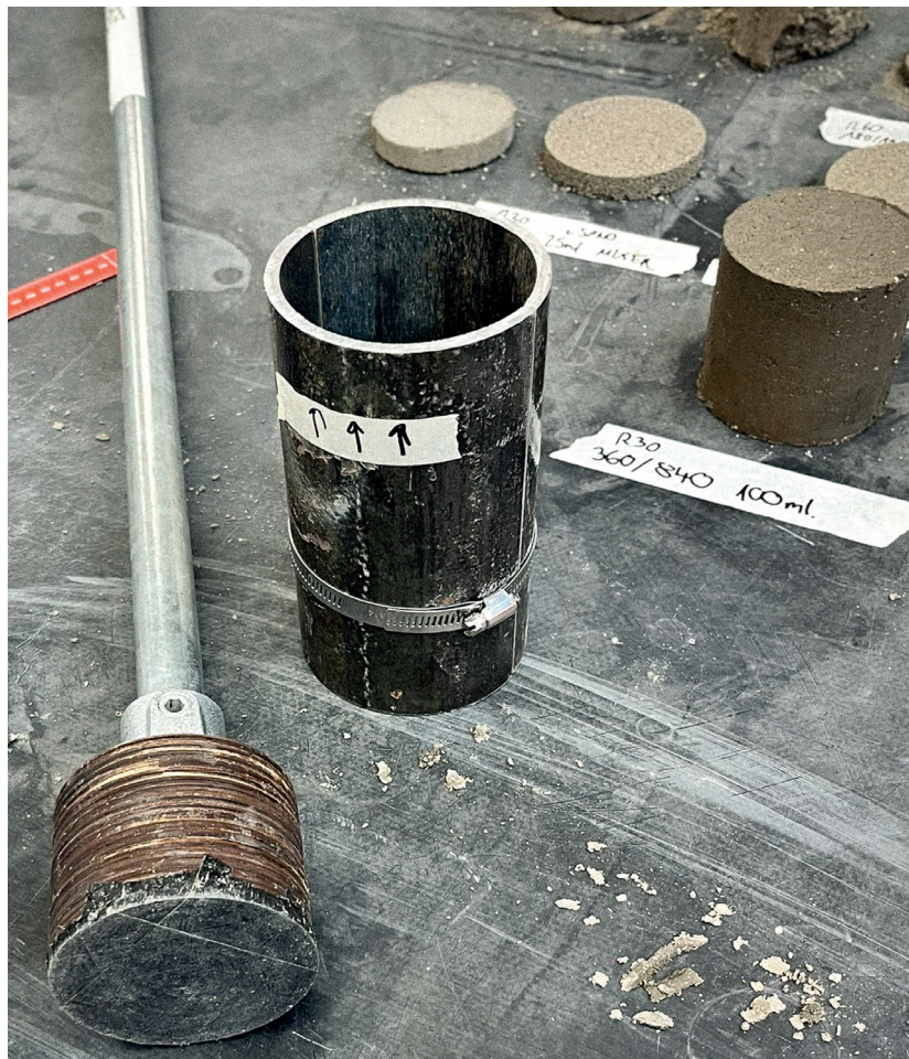
Figure 61: Experimental setup for dynamic compaction, showing the tamper and the split steel tube secured by threaded steel clamps.
