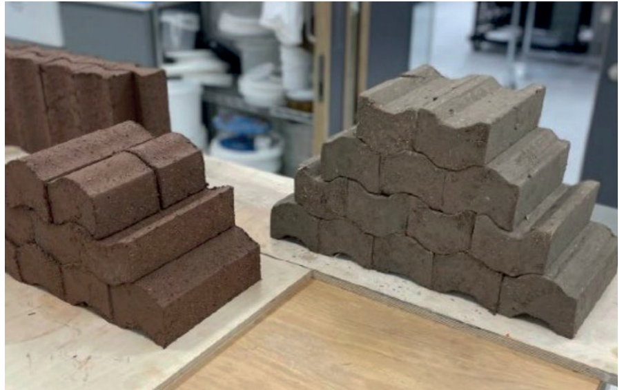
Figure 112: Exploratory interlocking earth brick prototypes developed by T. Jorgensen within the framework of extrusion-based manufacturing. Reproduced from Jorgensen (2023).
