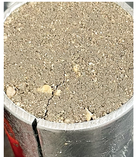
Figure 74: Crack formation at the tube opening.
