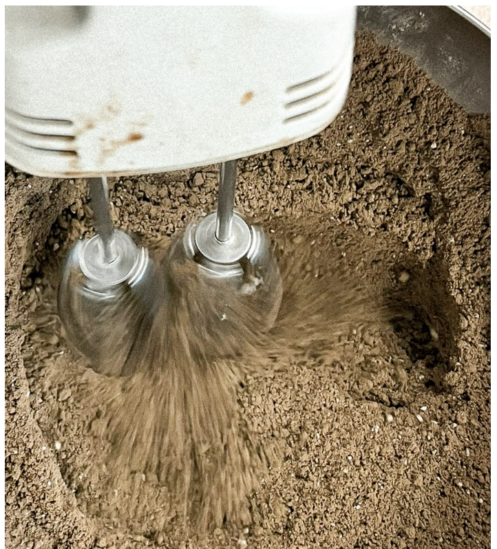
Figure 56: Homogenisation of the material using a conventional kitchen hand mixer.
