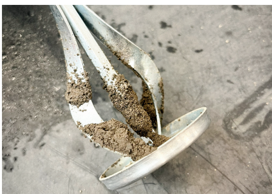
Figure 55: Adhesion of the material to the drill-mounted mixer.
