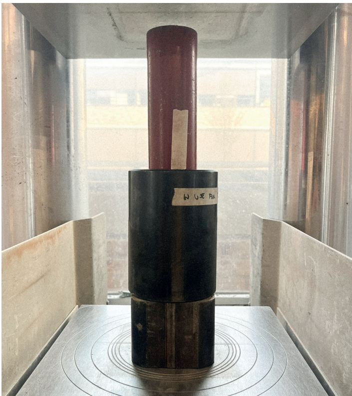
Figure 67: Demoulding setup with a hollow steel section positioned beneath the mould for specimen ejection.
