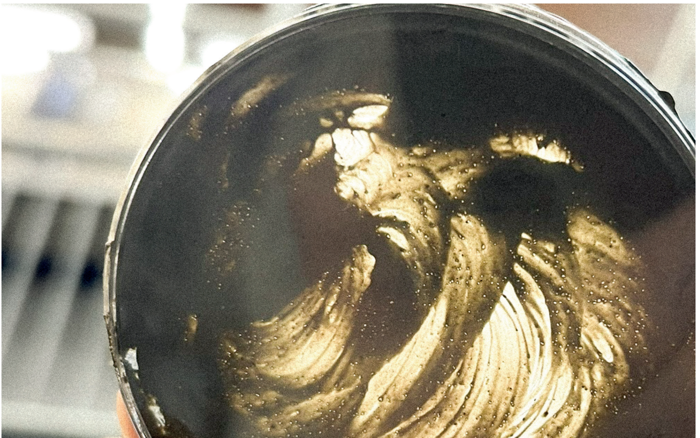
Figure 14: Fine granular fractions of the investigated material examined in a Petri dish against transmitted light.
