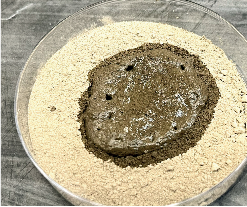
Figure 12: Natural carbonate assessment using 10% acetic acid solution, showing strong and sustained effervescence.
