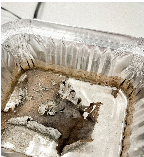
Figure 19: Oven-drying of the sand fraction retained on the 0.063 mm sieve
