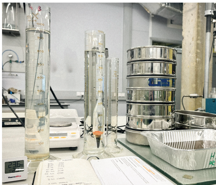
Figure 20: Hydrometer test setup with three graduated cylinders: soil suspension, reference solution and distilled water for meniscus correction.
