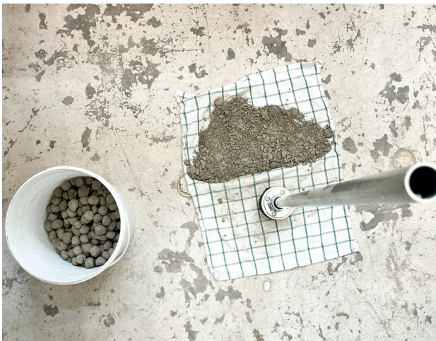
Figure 51: Mechanical pre-crushing of the dried material using a tamper.
