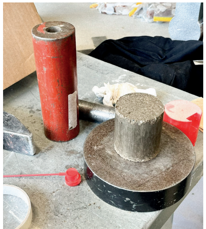
Figure 66: Compacted specimen after ejection from the mould.
