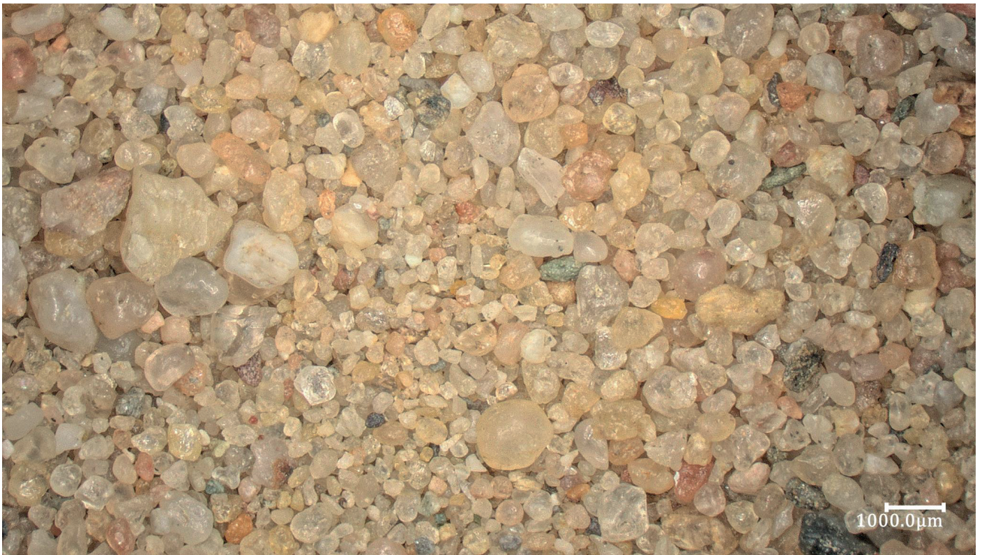
Figure 37: Microscopic view of the crushed sand selected for the mix design, captured using a 100 mm lens.
