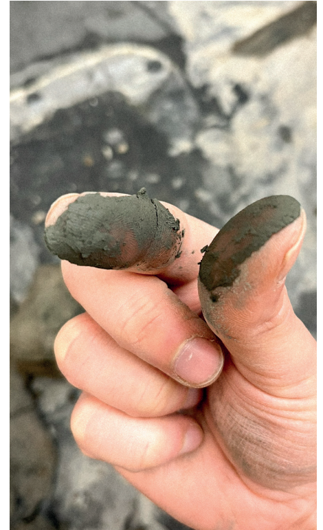
Figure 16: Texture assessment of the earth-moist material, indicating a cohesive, slightly sticky and rubber-like consistency.
