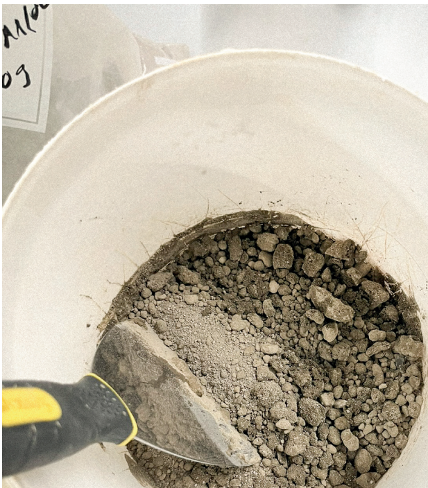
Figure 53: Clump formation during manual mixing trials.
