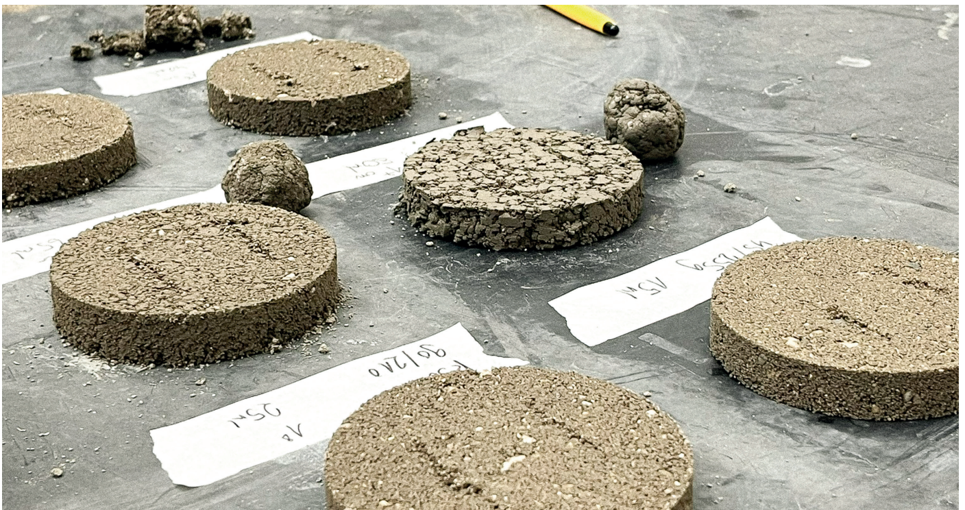
Figure 60: Pancake specimens with central grooves incised for shrinkage measurement.
