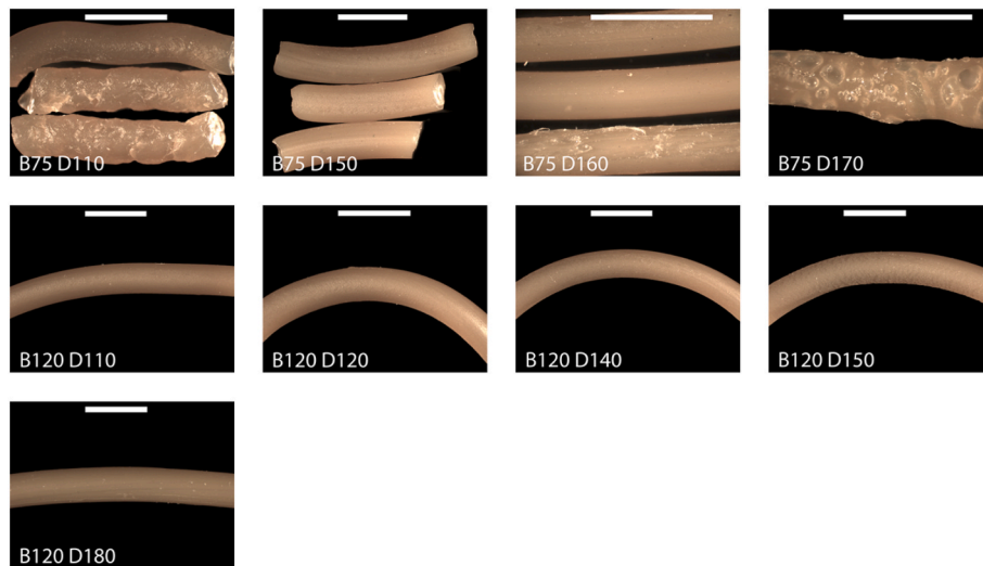
Fig. 12. Extrudate strand surface finish as a function of barrel (B) and die (D) temperatures ( ^{\circ}\text{C} ) for PHBV gel processing (Table 1). White bar scale indicates 5 mm.
