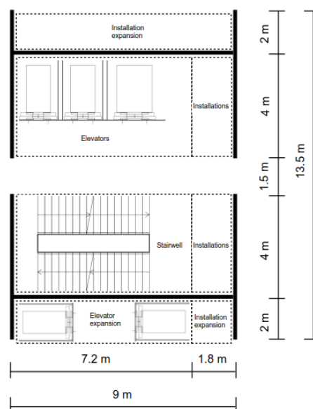
Figure 40: Smallest possible adaptable core lay out.
