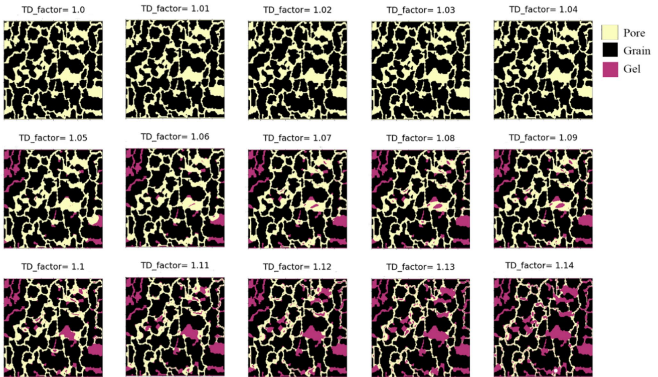
Fig. 10 Formation of gel in the pores of the Berea sample with different values for TD_factor
