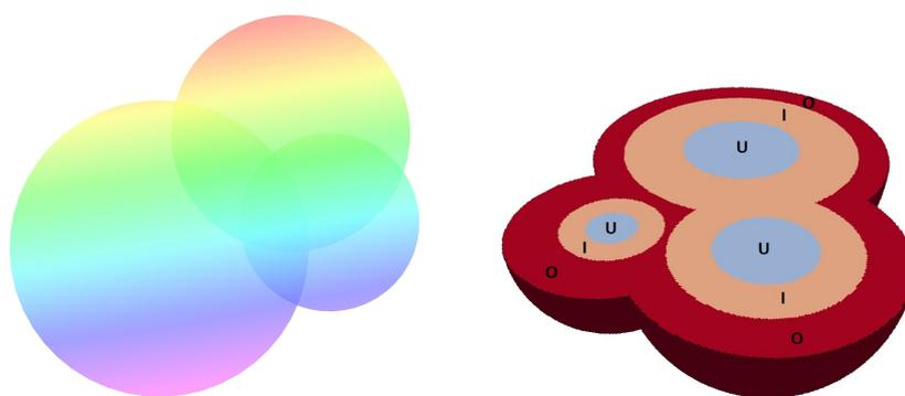
**Figure 3.3:** Contact of hydrating cement particles
