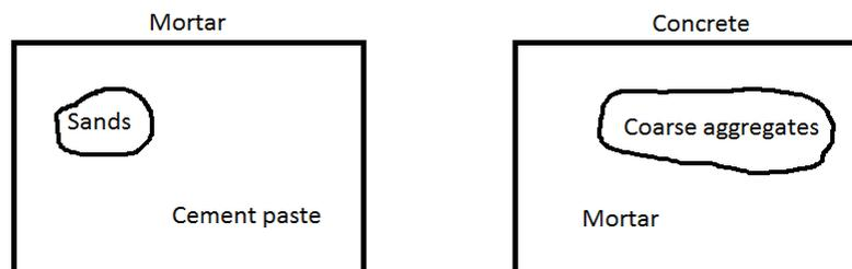
**Figure 4.1:** Cement paste, mortar and concrete
