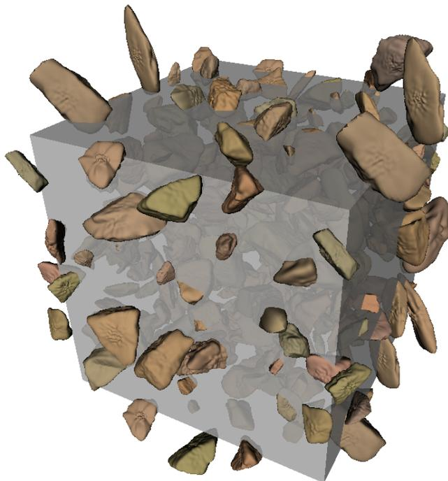
**Figure 4.12:** The mesostructure of the mortar specimen with irregular shape sand particles
