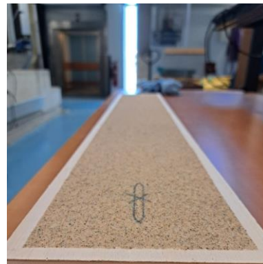
Figure 80 – The used plank with sand wood-glued on it
