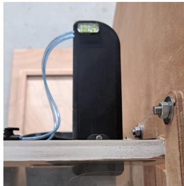
Figure 47 – Using a mini-level to place the pitot tube parallel to the flow
