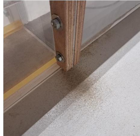
Figure 57 - Additional sand losses were spotted at transitions (this is from a few tests)
