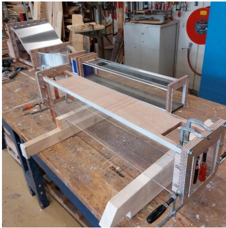
Figure 51 – Constructing the mobile wind tunnel system
