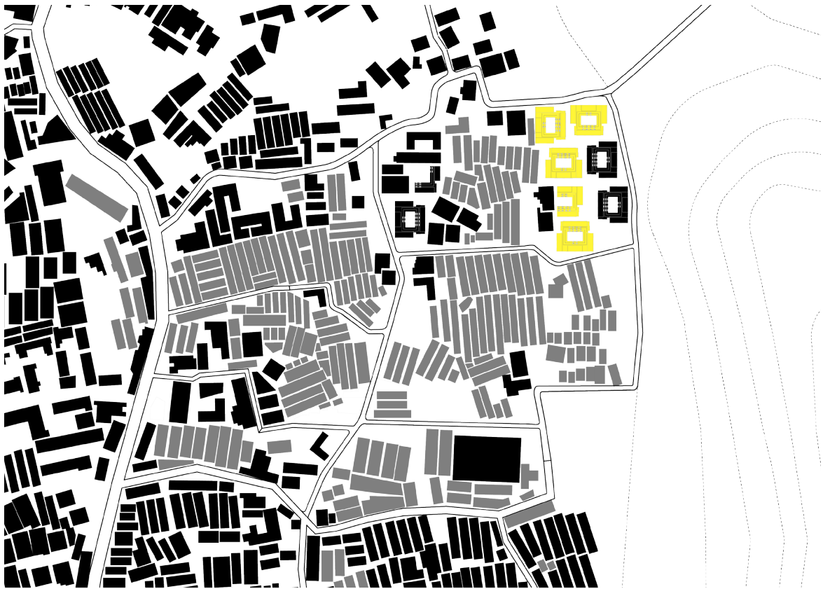
Step 4 move existing residents into finished blocks, sell the rest units, and start building new blocks
