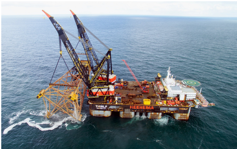
Figure 1.3: SSCV Thialf with the Jacket [28].
