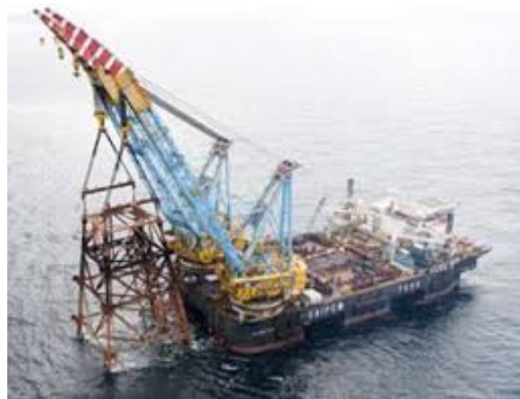
Figure 1.5: Frigg QP jacket on wet transport [3].
