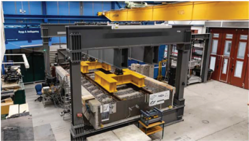
Figure 5. View of the full-scale trough bridge tested at the LTU lab.
