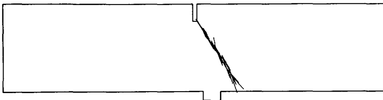
Figure 5.3 Single-edge-notched beam. Active cracks at final load.
