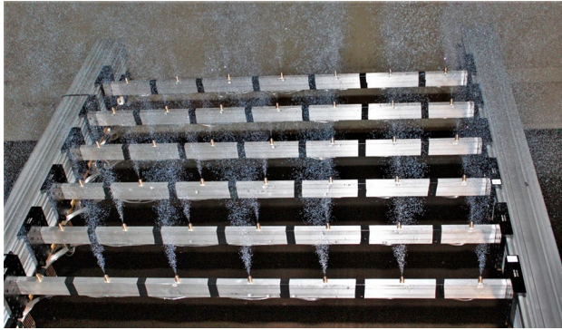
Fig. 15 NLR's seeding rake of 42 bubble generators
