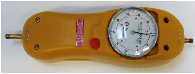
Fig. 12. Pull/push gauge 50N used for torque and force measurement of control box
