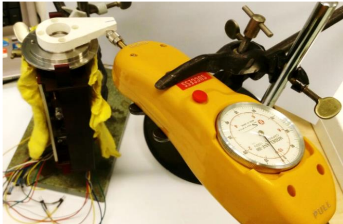
Fig. 17. Vertically clamped control box and the ANF-50 pull/push gauge for test setup of test 6
