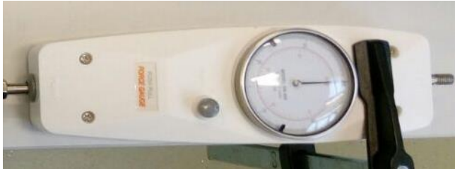
Fig. 13. Pull/push gauge 100N used for the force measurement of ZTM
