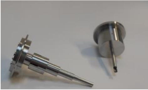
Fig. 2. CBC and IC pieces for coupling the control box and the SATA instrument
