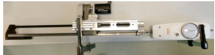
Fig. 19. Side horizontal fixation of the ZTM for test setup of test 2
