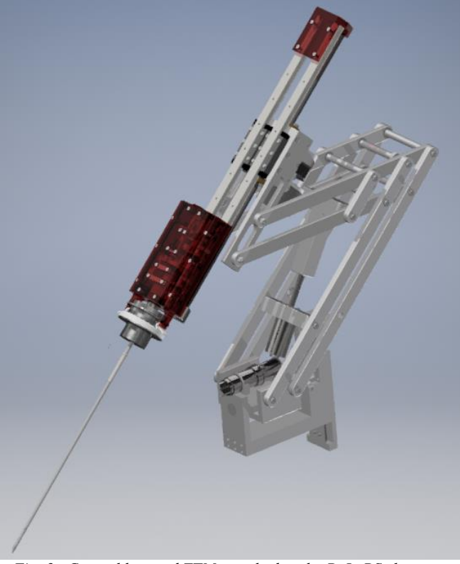
Fig. 3. Control box and ZTM attached to the PoLaRS slave arm
