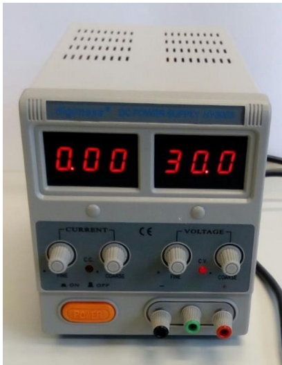
Fig. 14. Power supply digimess® DCPOWERSUPPLY HY3003 0-30V, 0-3A used to supply power to the control box
