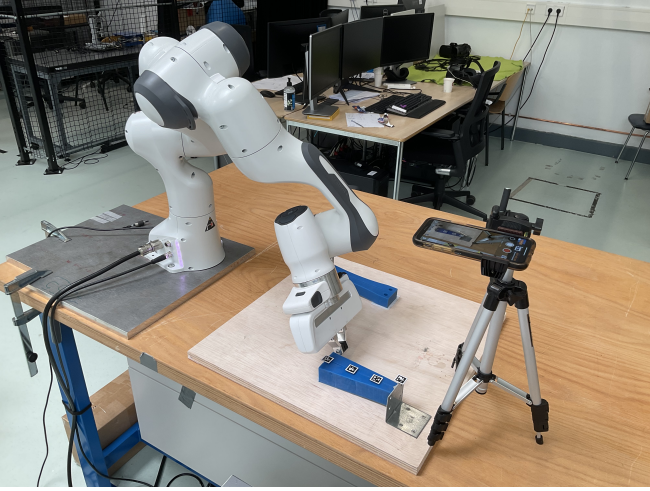
Fig. 2: Experiment setup. Visible are the Franka Emika Panda robot, the silicone beam, and the recording device attached to a tripod.
