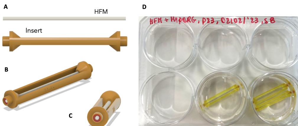
Figure 6.2: (A) The two components necessary for seeding cells are an HFM and an HFM chip insert. (B, C) The HFM is glued into the insert by means of a biocompatible dental glue (red). The inner compartment of the insert should be completely filled with dental glue. (D) After gluing and seeding of cells, inserts could be kept in a six-well plate in the incubator for culturing.
