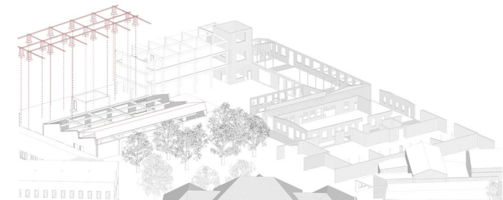
Intervention building 3: Extension to the side; new walls made out of reclaimed brick. New function: Public workshop
