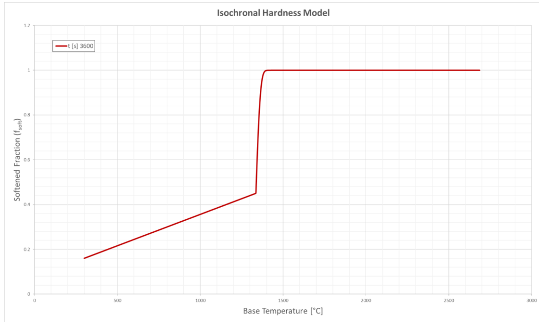
Figure 90. Tungsten softening expected behavior after 1 hour for the 300 – 2700 °C range
