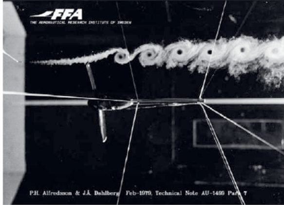
Figure 1.10: Smoke visualisation of vortices being shed at the tip of a wind turbine rotor 12 .
