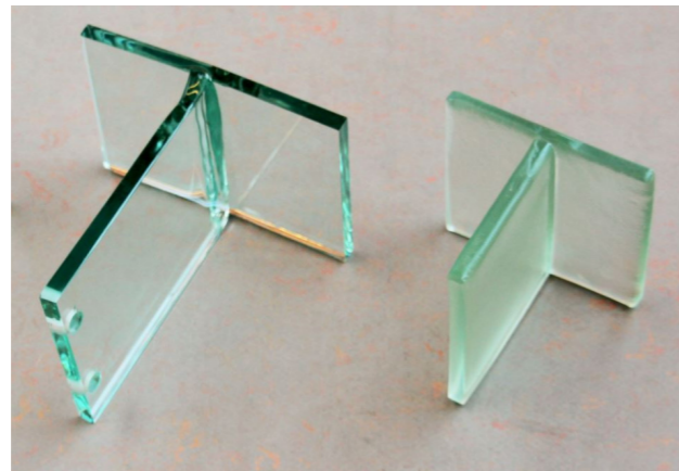
Figure 12: Welded Glass (Left) & Fused Glass (Right) | Source: Eskes, 2018
