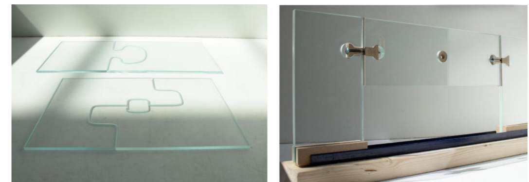
Figure 14: Interlocking glass profiles | Source: Bouwmeester (2023) (left) & Motedayen (2025) (right)
