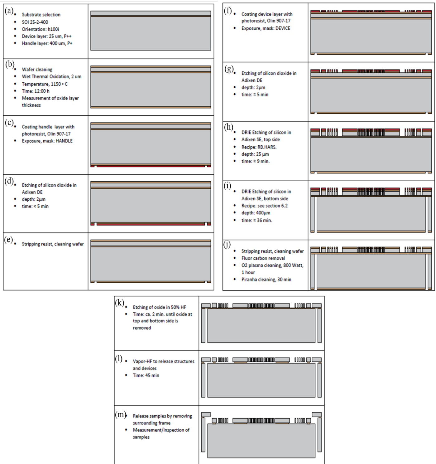
Figure 20: Fabrication Process Sequence at MESA+ Lab
