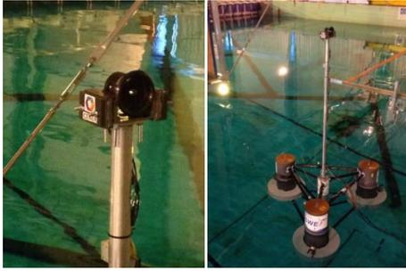
Figure 3.28 Ducted-fan-based FOWT test [45]
