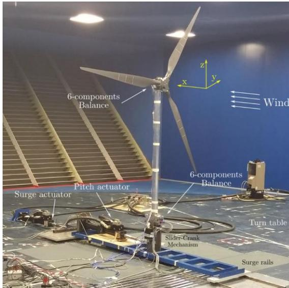
a. Wind tunnel test setting
