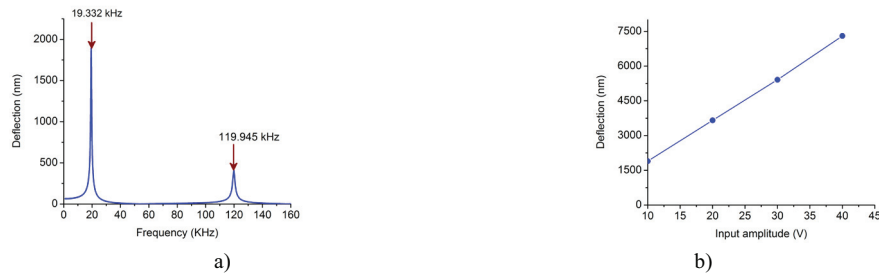
Fig 6: First and second resonant frequencies of the slender 50 \mu\text{m} wide and 200 \mu\text{m} long cantilever (a) and dependence of the measured deflection on input amplitude at first resonant frequency (b).
