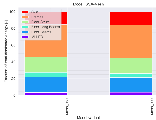
Figure 8.3: Energy absorption distribution by component, mesh sensitivity analysis. No significant variations are noted, for different mesh refinement levels. The '080' and '090' values denote a global element size equal to 0.80x and 0.90x that of the baseline, respectively.
