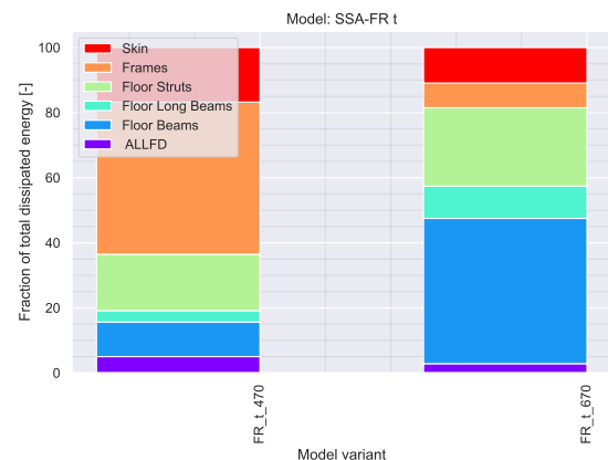
Figure 8.14: Energy absorption distribution by component, frames thickness sensitivity analysis. The frames' bending stiffness has a significant impact on the energy-absorption characteristics of the section.
