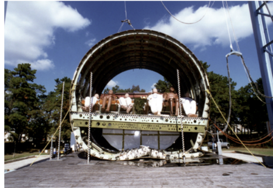
Figure 3.8: Post-crash of Boeing 737 typical fuselage section, with an auxiliary fuel tank onboard [30].
