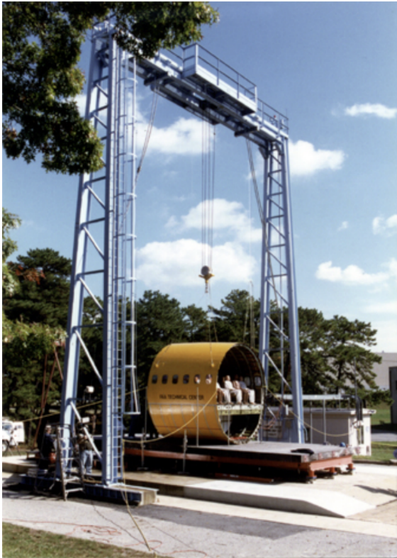
Figure 3.7: Boeing 737 typical fuselage section drop test setup [30].
