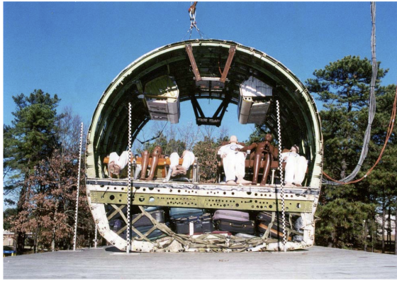
Figure 3.9: Boeing 737 typical fuselage section drop test, with luggage in the cargo bay [31].
