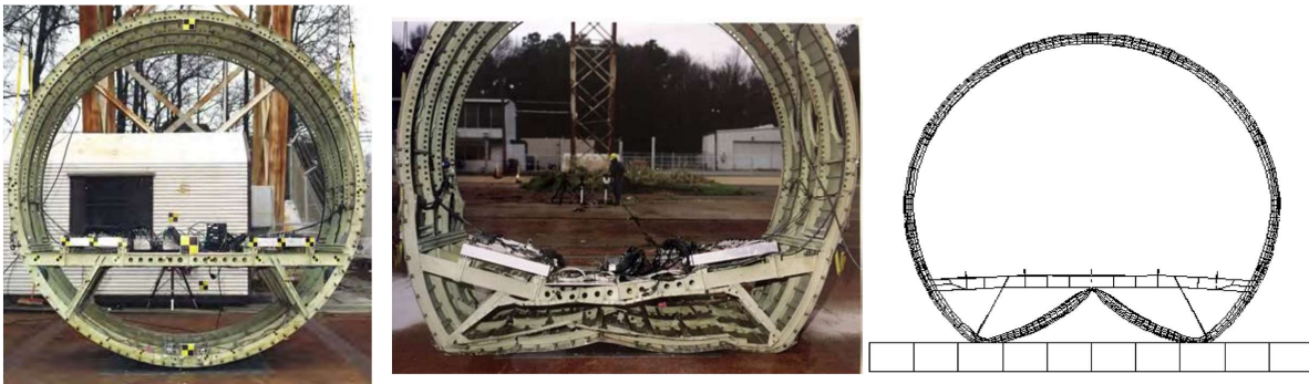
Figure 4.3: From left to right: pre-test, post-test, and simulation results from the F-28 drop test performed at NASA LandIR; adapted from [37, 39].
