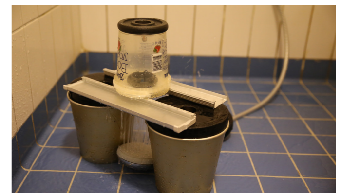
I.4. Drain element sprayed with showerhead
