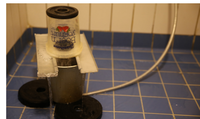
I.3. Drain element sprayed directly with tap water
