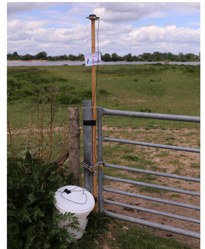
8.2. Temporary base station setup at the Broomwaard.
