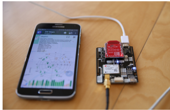
6.5. Android phone running SWmaps, connected to ArduSimple GNSS receiver using Bluetooth
