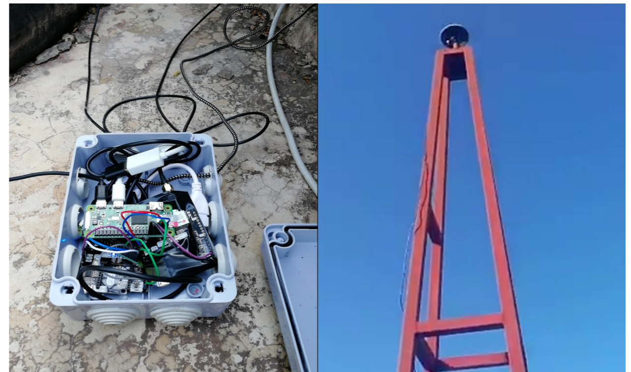
image / figure 2: Current state of the base station; left: the electronics, right: its fixed location antenna
