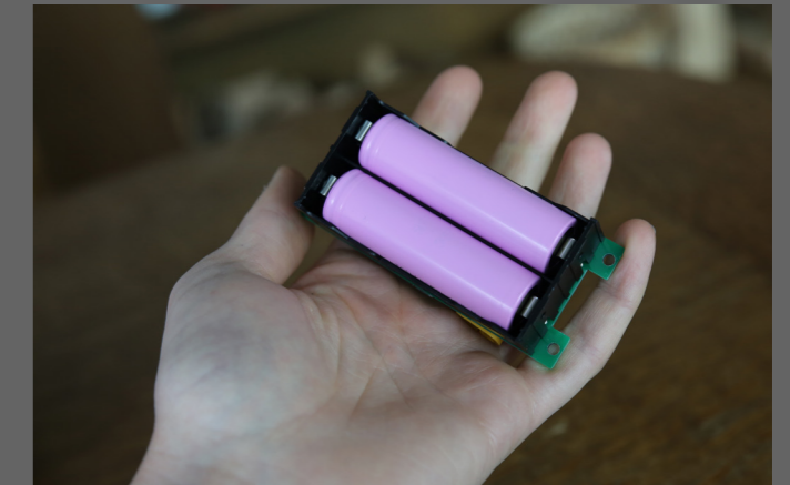
6.41. Rover battery lithium-ion cells.
