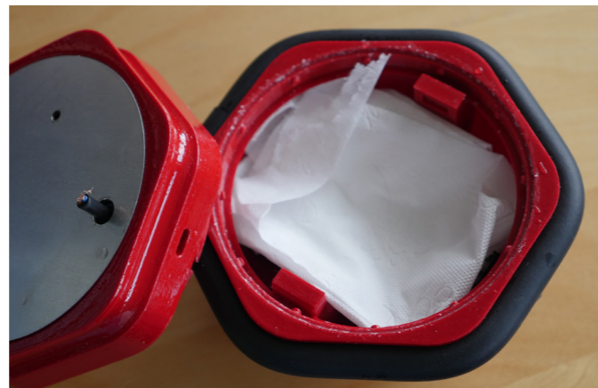
6.24. Tissues within the device are dry after 15 minutes of rain.
