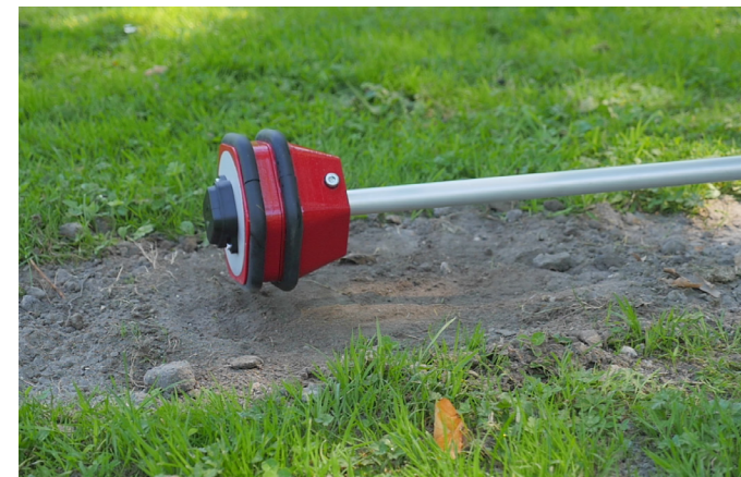
6.44. ROVER2 model undamaged after fall on sand
