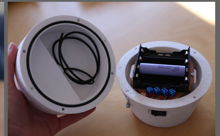
6.20. ROVER1, O-ring in a groove which can be tightened with 4 bolts
