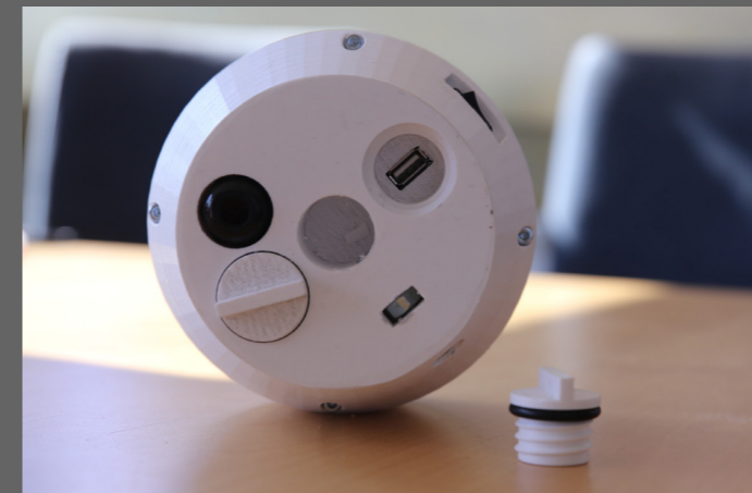
6.19. ROVER1, plugs to close off usb ports
