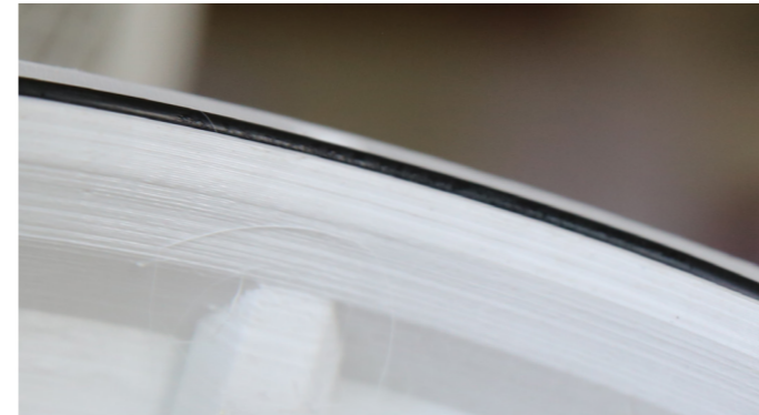
J.3. Visible moisture on O-ring
