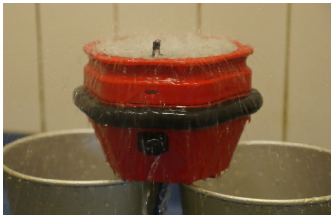
6.23. ROVER2 in the 15-minute rain test using the shower.
