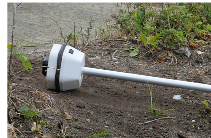
6.42. In between rover model has slight internal damage after fall on sand.
