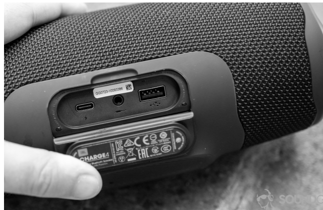
6.17. Connectors of JBL charge 4 can be closed off using a plug.
