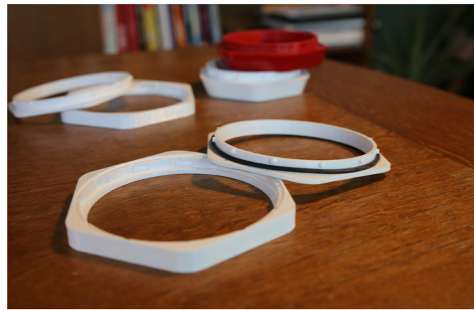
6.22. Test models of the 12-notches seal mechanism
