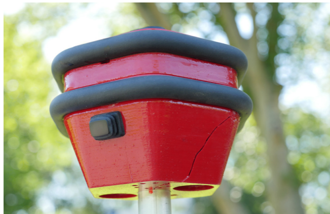
6.46. ROVER2 lower rover housing cracked after fall on asphalt.
