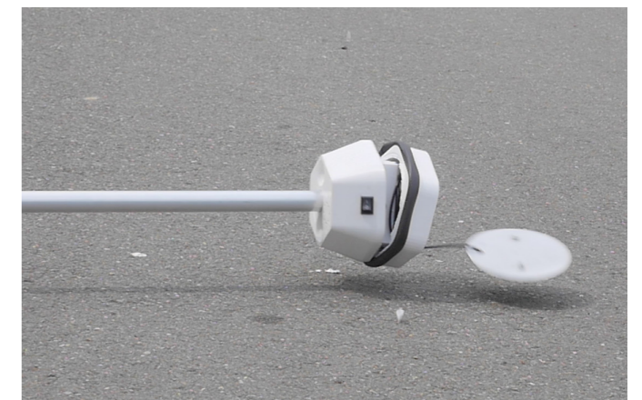
6.43. In between rover model collapsing after fall on asphalt
