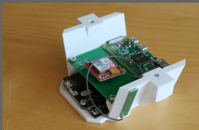
6.30. Sim800L and antenna on BASE1 electronics rack.
