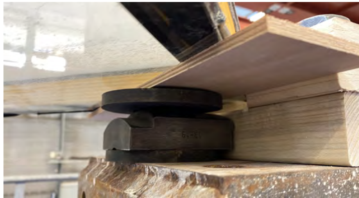
Figure 4.8: Support for the 4 mm panels. A steel block with a rounded top, a thick rubber pad and a piece of multiplex created a flexible support to spread the load.
