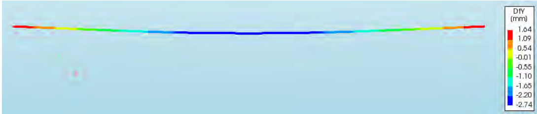
(b) Vertical displacement plot of the model. Scale factor = 1. The colour scale runs from -2.74 mm (blue) to +1.64 mm (red).
