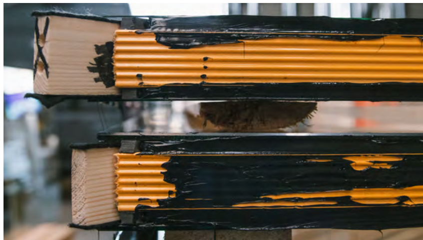
Figure 4.19: Comparison between the 1.1 mm CT glass (top) and the 4 mm FT glass (bottom).
