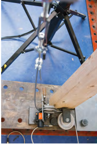
(a) Full view of the load cable, pulleys, LVDT sensor and the wire gauge attached to the panel's corner.
