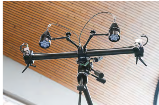
Figure 4.14: The GOM ARAMIS Adjustable camera system used for the 3D digital image correlation.
