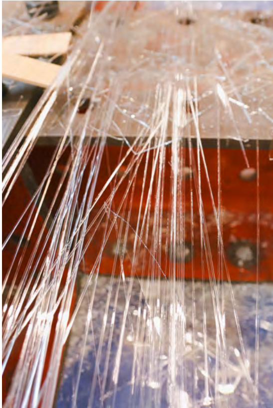
Figure C.14: The glass spaghetti-like rods resulting from the fracture of the top plate of the 1.1 mm panel.
