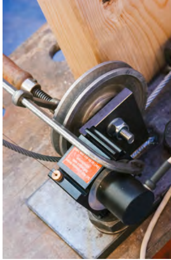
(b) The LVDT sensors were clamped to the pulley so that the wire gauge came out as close to the cable as possible.
