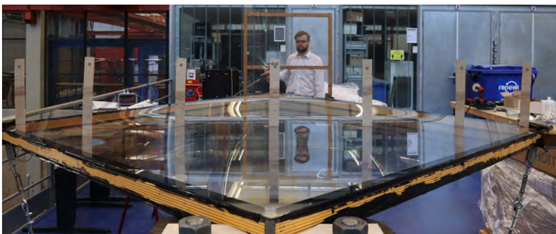
Figure 4.28: In the first deformation stage, where the loaded diagonal was fairly straight and the supported diagonal was curved.
