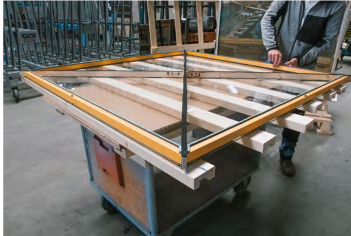
Figure 4.20: The first panel, partly assembled on the movable cart. Note the orange GFRP profiles that form the frame. The spacer tape is placed on the inside edges of the frame, lengthwise as well as in the corners. The blue film to protect the spacer tape's adhesive is removed before placing the top panel. The removable timber cross can also be seen here.
