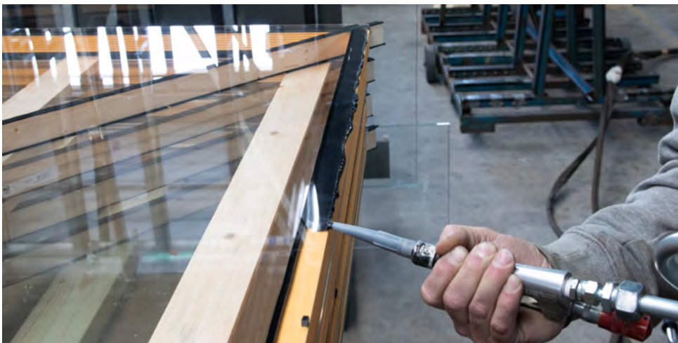
Figure C.3: D993 silicone being applied
