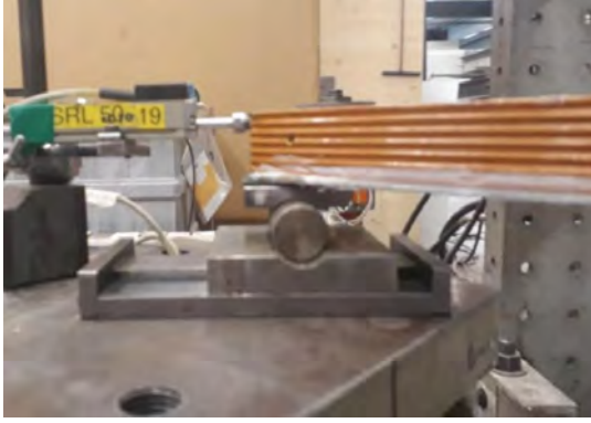
Figure 4.3: One of the roll supports used in the experiments by Young (2019).
