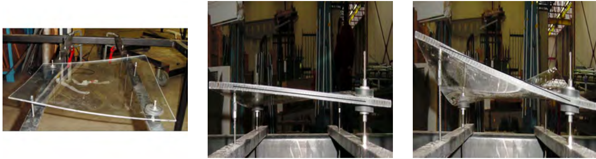
(a) The setup consists of a polycarbonate plate supported at all four corners. Two corners are held in place, while the other two are pushed upward.
