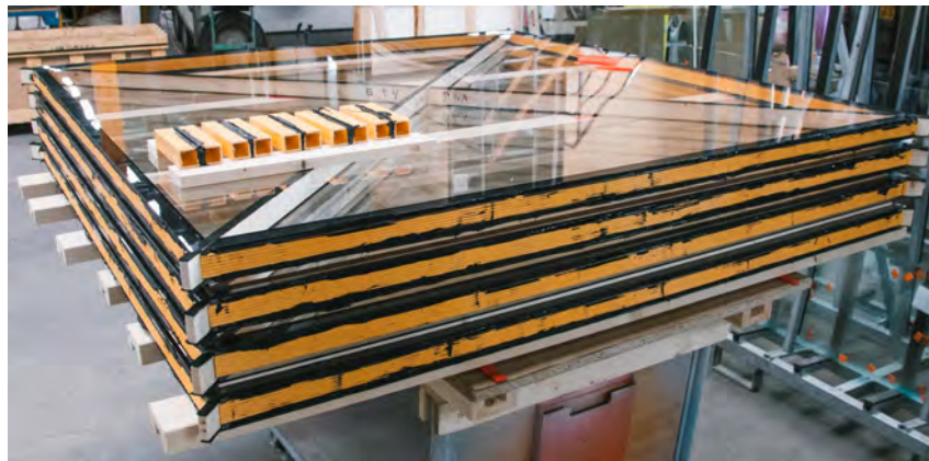
Figure 4.22: The full stack of assembled panels. The bottom three panels are with 4 mm glass, the top one is with 1.1 mm glass.
