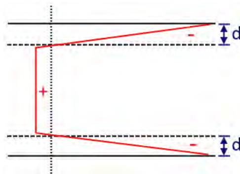
Figure 2.13: Schematic stress profile of chemically toughened glass. Case depth d (usually very small compared to the full glass thickness) is the depth at which the prestress reaches zero.
