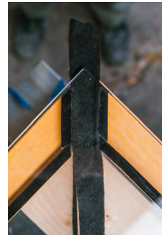
Figure 4.21: Top view of the corner of one of the panels. Note the orange GFRP profiles with the black spacer tape on the inside edge and the timber cross with black felt through the middle of the image.
