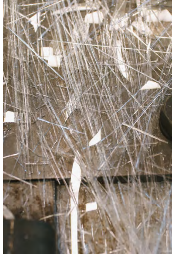
Figure C.15: The glass spaghetti-like rods resulting from the fracture of the top plate of the 1.1 mm panel, along with the larger shards of the bottom panel.
