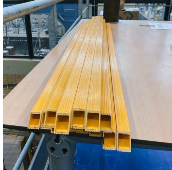
Figure 4.18: The GFRP profiles cut to the correct length of 1.48 m, with 45° angles at both ends.
