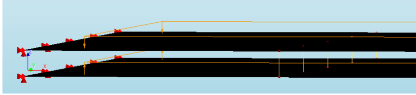
Figure 3.17: DIANA model used to test springs as a way of modelling contact between plates.
