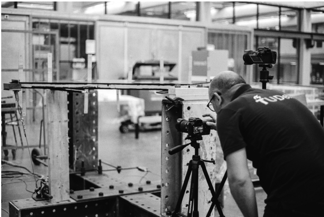
Figure C.10: Setting up the 2D DIC cameras, one for the top plate, and one for the bottom. Image shot on 35 mm black-and-white film.
