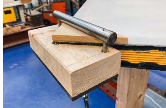
Figure 4.24: Corner detail with MDF triangle to spread the load.
