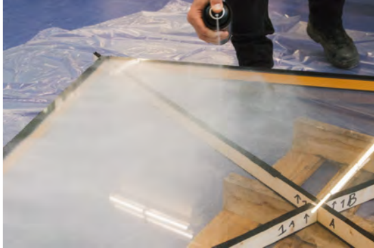
Figure 4.23: The white base layer of rubber paint being applied.
