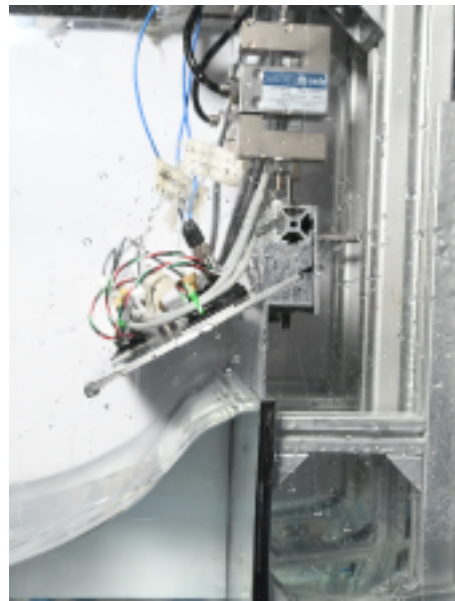
(c) Incoming wave impact on thick 4.0 mm plate instrumented with multiple, different pressure sensors. Zemic H3 50 kg reaction load cell at the top.
