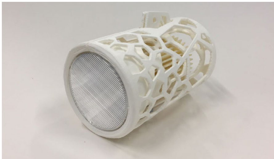
Figure 15 A 3D printed example showing the complex geometries possible with a low-cost 3D printer.
