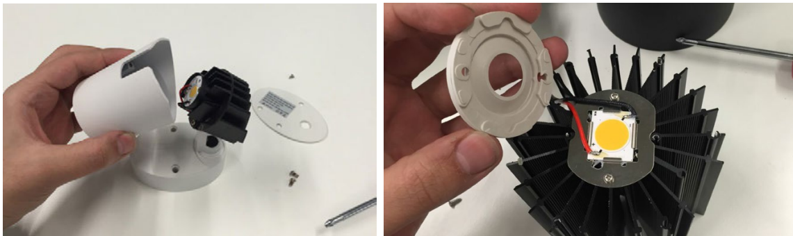
Figure 2 Two of many photos showing the reverse engineering of existing track downlights used to better understand the internal componentry.
