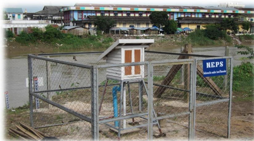
Figure 6.8.1 Automatic water level gauge station – Bago City – Bago River – Owner: Japanese researcher – This is not a station of DMH. - Photo: Rens Hasman
