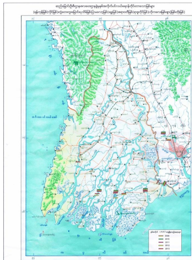
Figure 7.10.7 Salinity map of the Ayeyarwady Delta – produced by Hydrology Branch, ID, MoAI. The coloured bars indicate the salinity threshold value of 1ppt during the lowest discharge of the Ayeyarwady (end of May during spring tide) for the years 2009 to 2013
