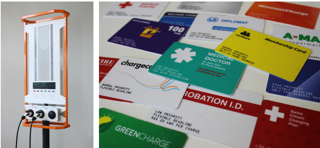
Figure 23: The first prototype of the transparent charging station and the ID cards based on which the system determines the charging priority (The Incredible Machine).
