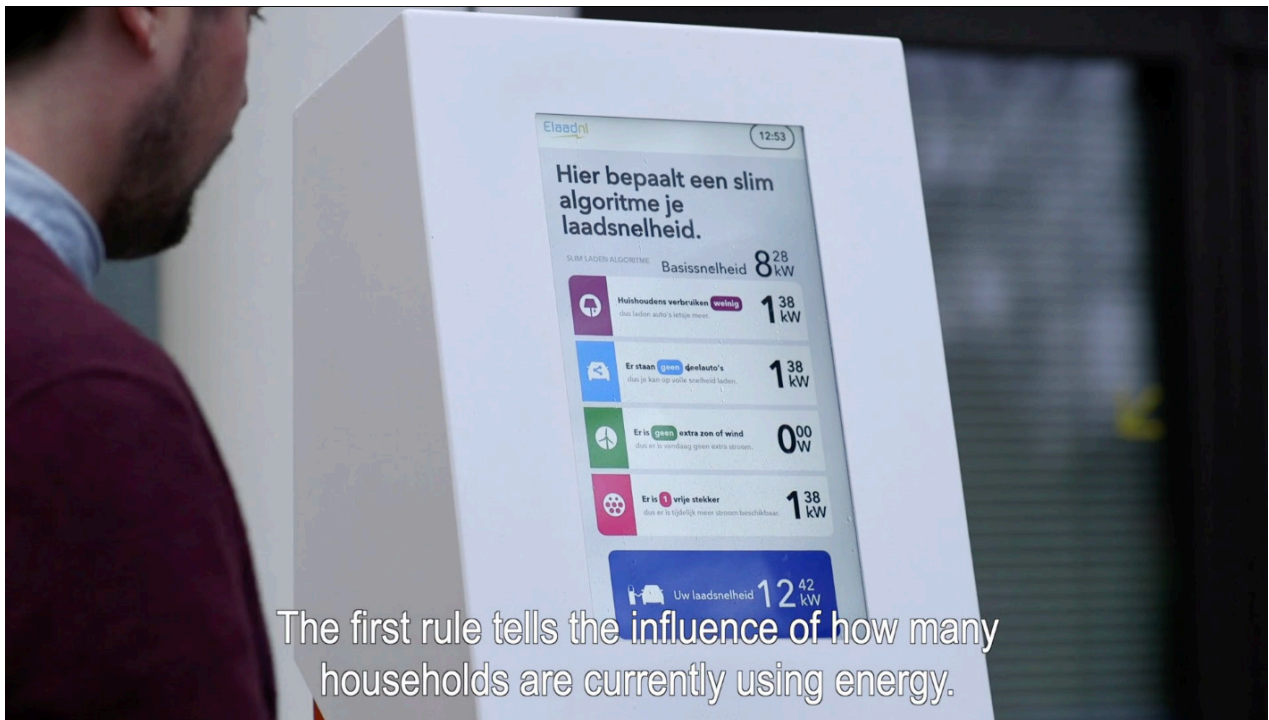
Figure 24: The second prototype of the transparent charging station makes the rules, which the smart system uses to determine the distribution of energy, visible to the user (AMS Institute).
