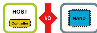
Figure 4.3: In a third and final configuration: a host itself can manage a flash memory, where the controller software is run directly from the main processor.
