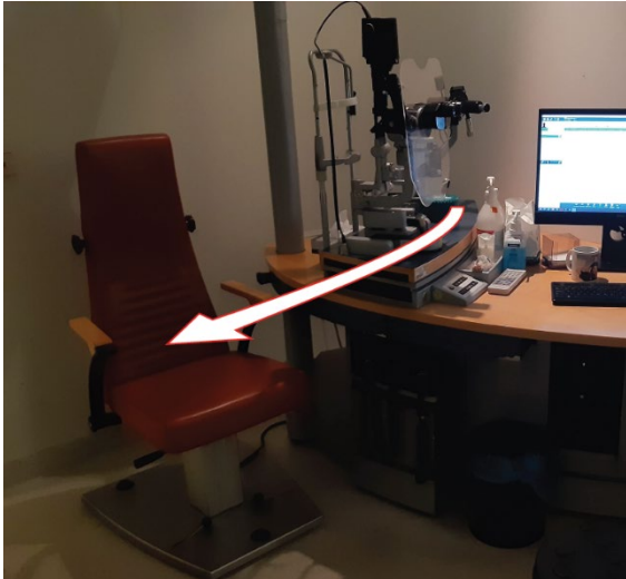
Figure 8-7: Ophthalmic table unit with Circular translation
