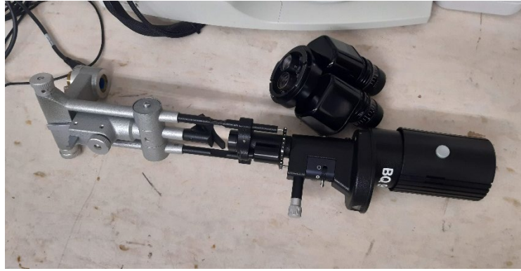
Figure 8-1: Slit Lamp eyepiece (back) and Lamp module (front)
