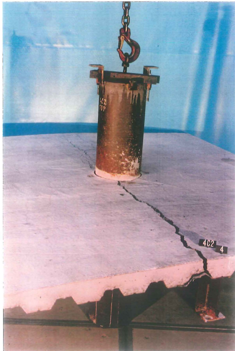
Photo 6-33 : Specimen 4C2 after failure
