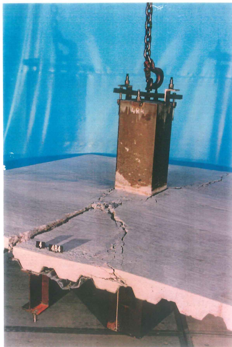
Photo 7-36 : Specimen 4R4 after failure
