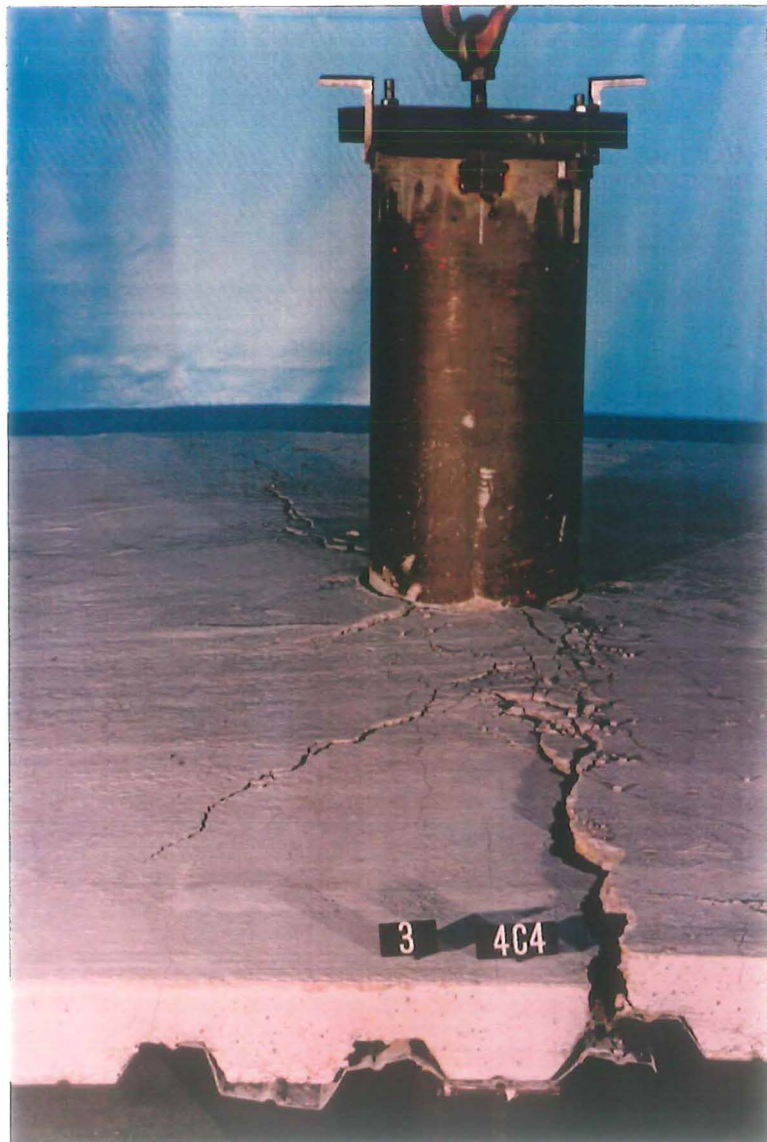
Photo 6-38 : Details of specimen 4C4 after failure
