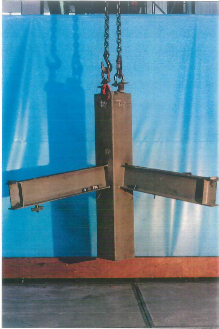
Photo 7-28 : Specimen 3R4 after failure
