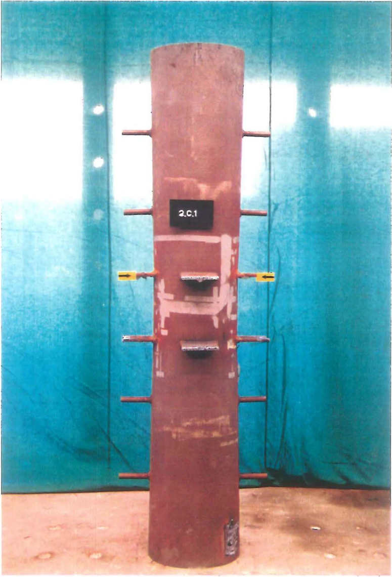
Photo 6-17 : Specimen 2C1 after failure
