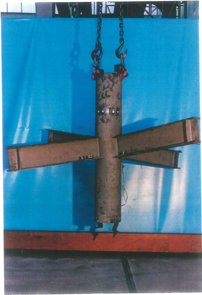
Photo 6-27 : Specimen 3C3 after failure
