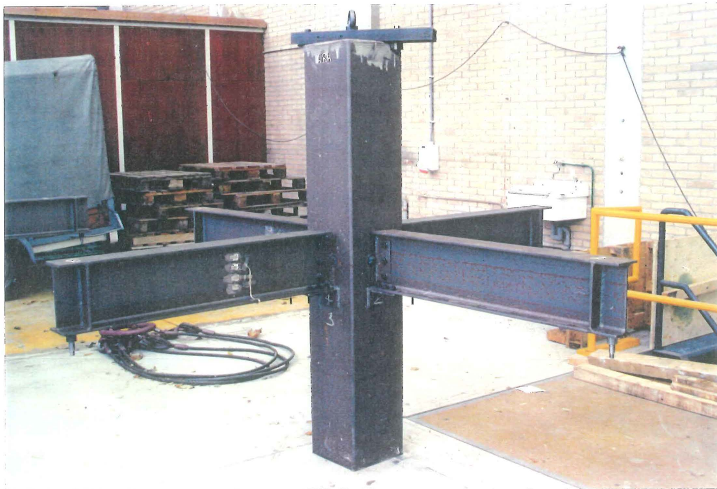
Photo 4-6 : Beams bolted to RHS columns
