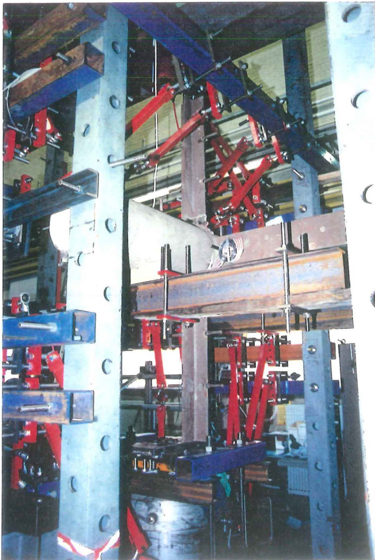
Photo 4-14 : Test rig for series 1 and 2, specimen 1C4, with composite CHS column and primary members (plates) in compression
