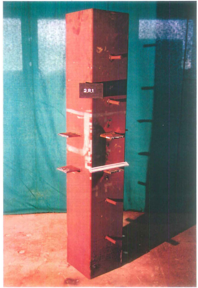
Photo 7-17 : Specimen 2R1 after failure
