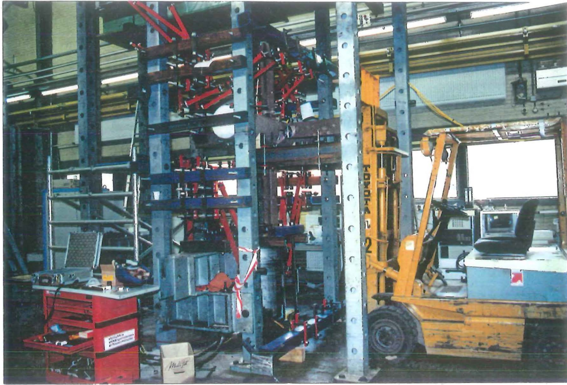
Photo 4-13 : Test rig for series 1 and 2, specimen 1C4, with composite CHS column and primary members (plates) in compression
