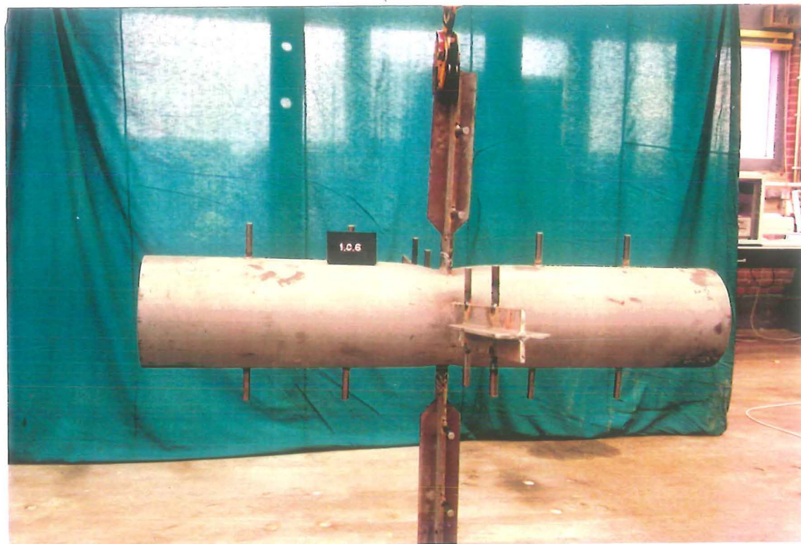
Photo 6-11 : Specimen 1C6 after failure
