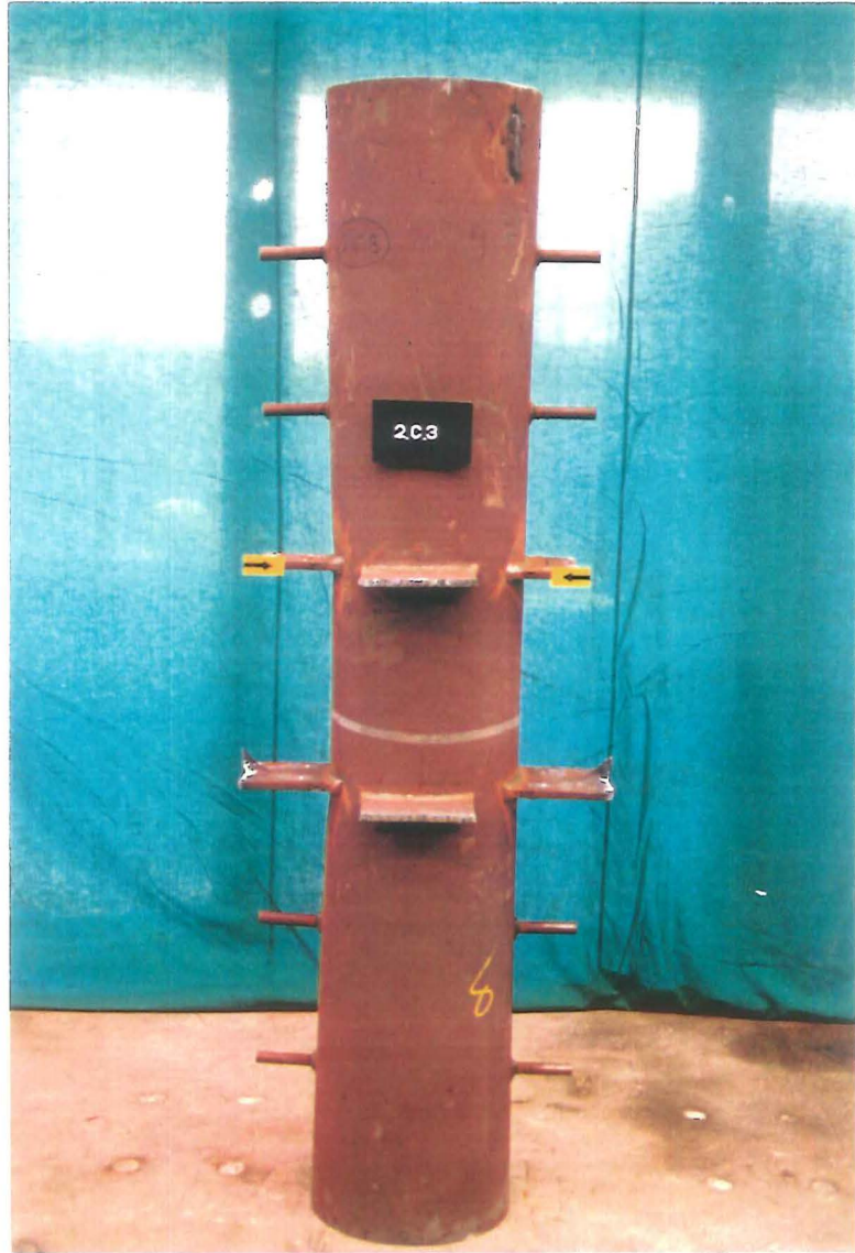
Photo 6-21 : Specimen 2C3 after failure
