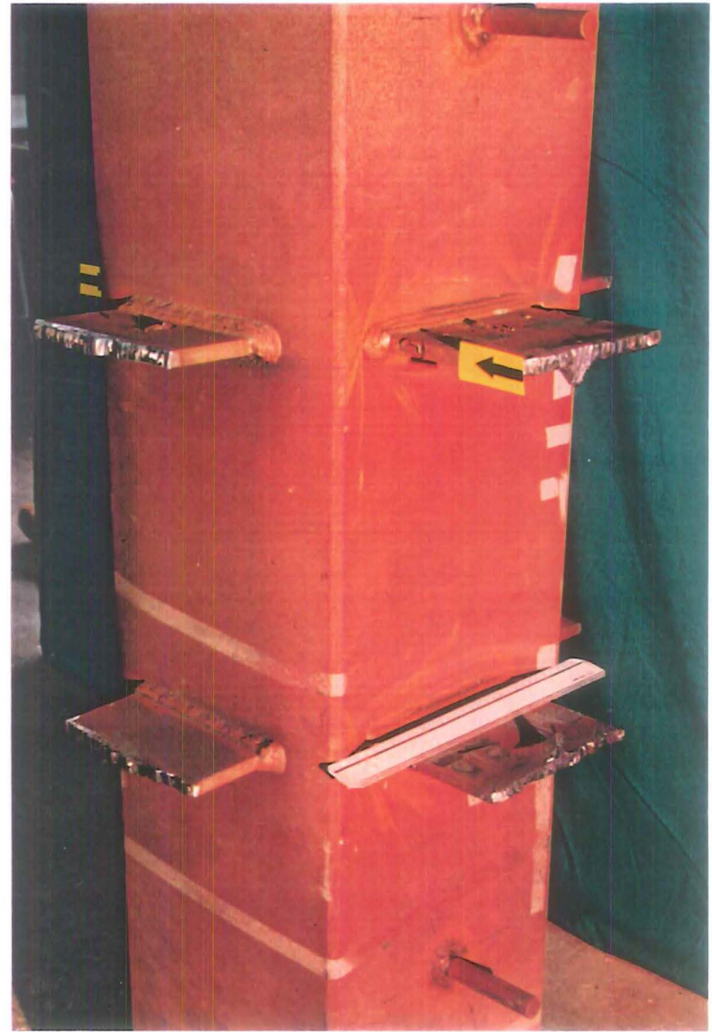
Photo 7-21 : Details of specimen 2R3 after failure
