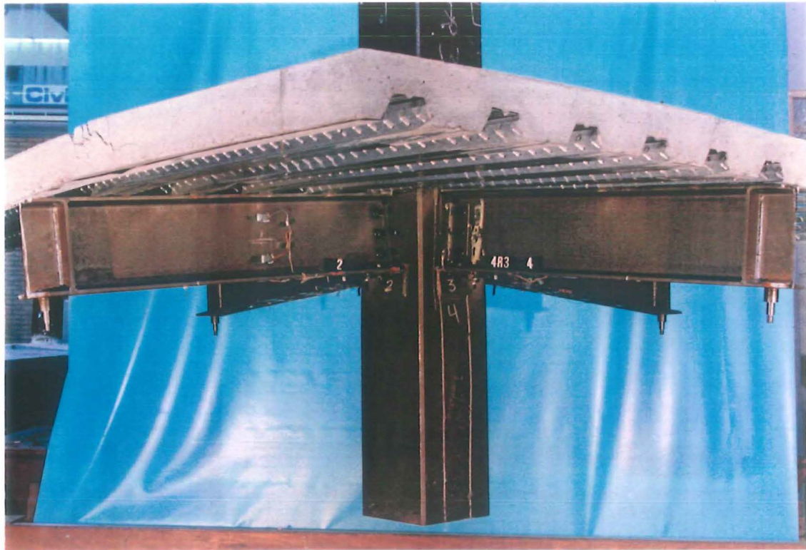
Photo 7-35 : Details of specimen 4R3 after failure
