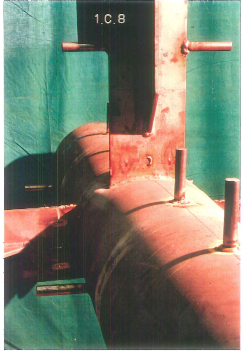
Photo 6-16 : Details of specimen 1C8 after failure
