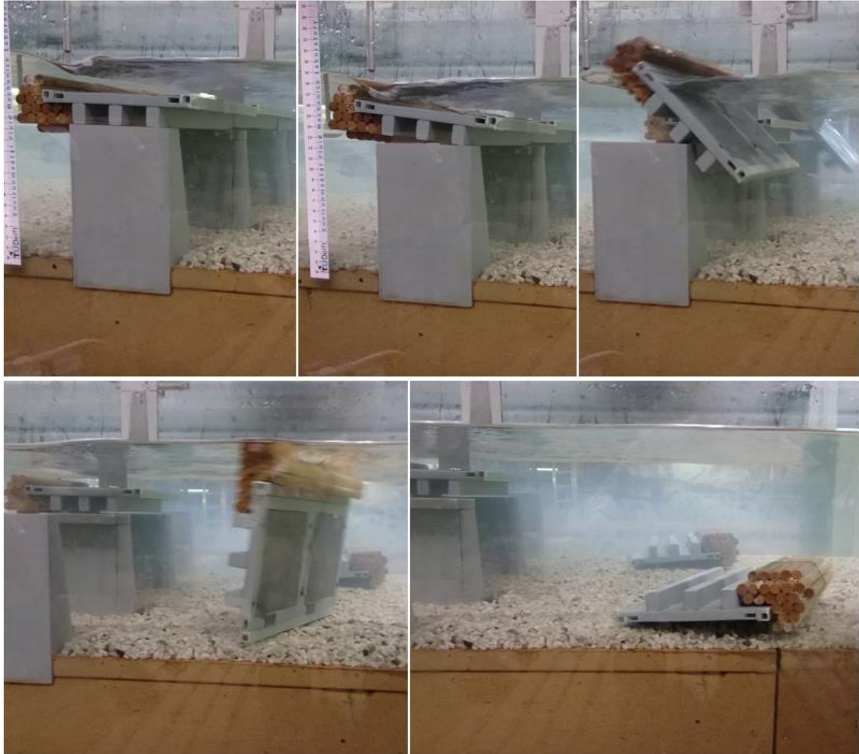
Figure 102: collapse of bridge deck with debris by overturning at relatively low flow velocities
