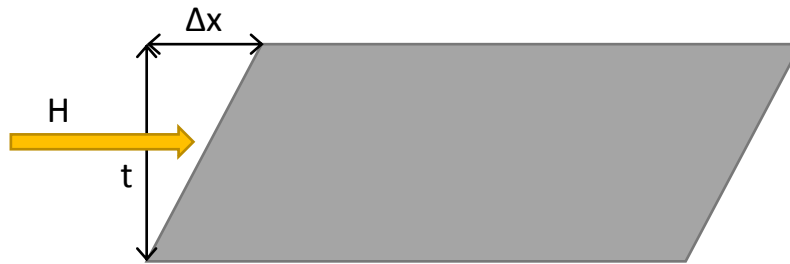
Figure 29: shear deformation \Delta x of an elastomeric pad with thickness t by a horizontal force H .
