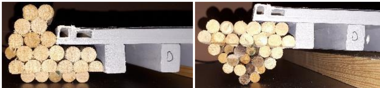
Figure 53: Side views of debris shape 1 (left) and debris shape 2 (right). Shape 3 (not shown here) is identical to shape 1, except it has cutouts in the front.
