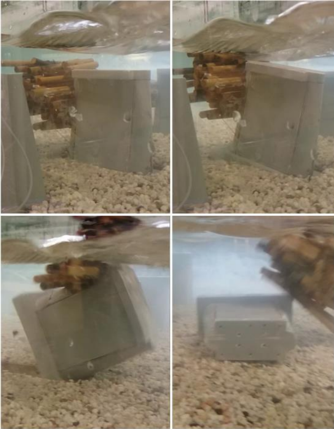
Figure 103: collapse of bridge pier
