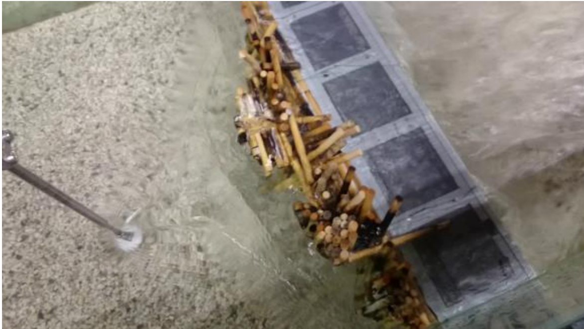
Figure 66: large amounts of simulated debris against the connected deck-pier system
