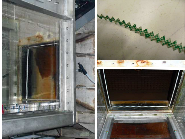
Figure 3.6: Left : Contraction with zigzag strips Right: (up) Close up of zigzag strip (bt) photograph of zigzag strip
