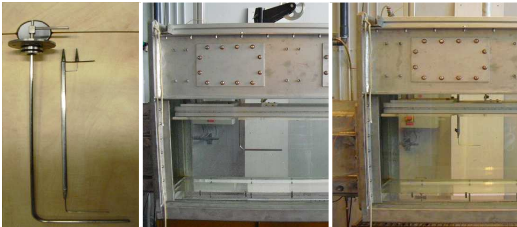
Figure 3.22: Left : Used Pitot tubes Middle: Large Pitot tube measuring U_\infty Right : Small Pitot tube measuring U_\infty
