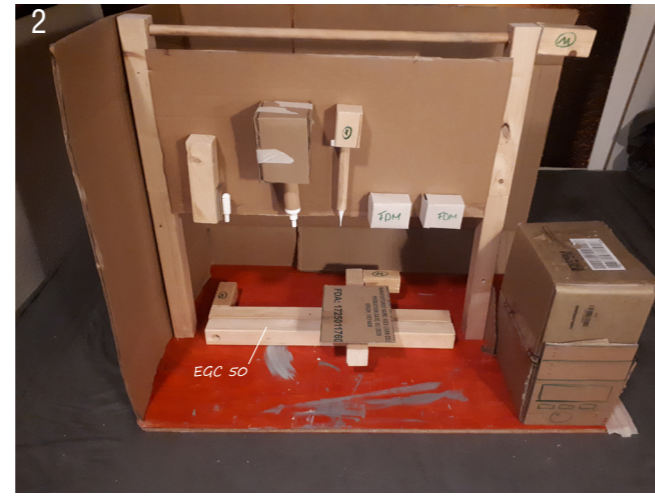
Instead of using double guides a bigger linear actuator is used for the X movement. For the Y-axis 600mm linear actuators are used.
