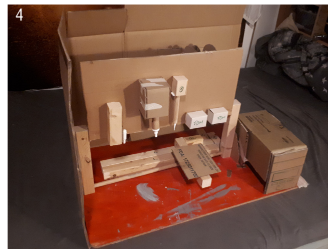
Instead of using double guides a bigger linear actuator is used for the X movement.
