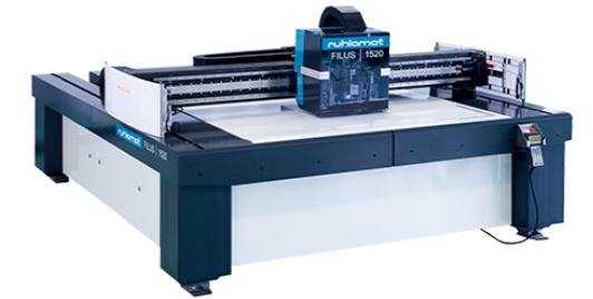
Figure 4.17 Ultra sonic wire embedding, soldering, pick & place
