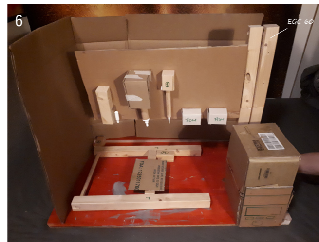
This setup also has the Z-axis in plane but uses a single bigger actuator for the Y-axis
