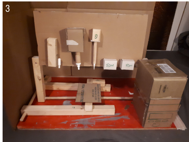
Setup with multiple drive axles and both the X and Y axis have double guides. The actuator and guides are placed so the axles won't interfere. Therefore longer x axis actuators are needed.
