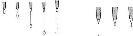
Figure 3. Dripping mode (left) and microdripping mode (right). (adapted from Cloupeau and Prunet-Foch) 2
