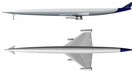
Figure 1: The LAPCAT A2 conceptual design
