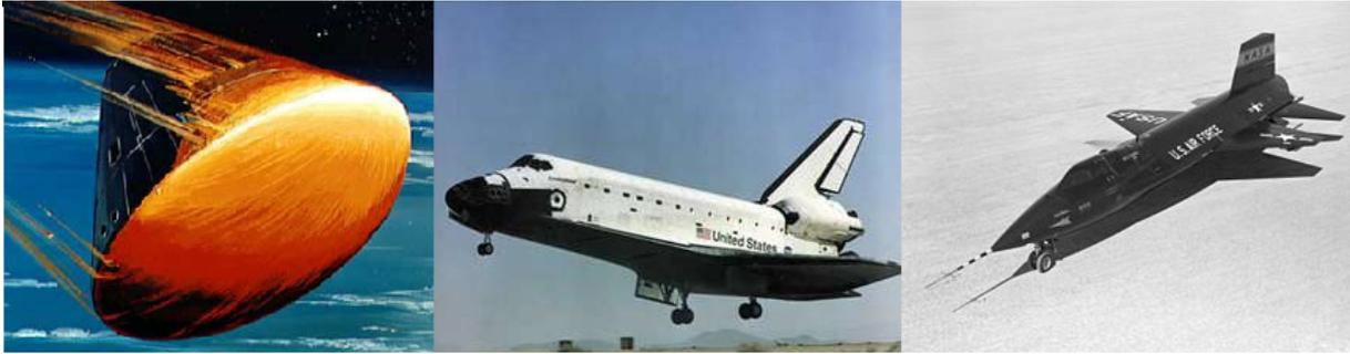
Figure 7: Types of Hypersonic vehicles; Left: Re-entry Apollo capsule (NREV) [113], Center: Space Shuttle (WREV) [47], Right: X-15 (CAV) [90].
